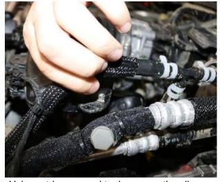
Using a trim removal tool, remove the clip securing the coolant hose to the factory air duct.
