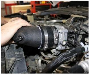
Install the straight sleeve onto the throttle body.
