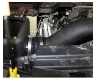
**8.** Install the air duct into the hump hose.
