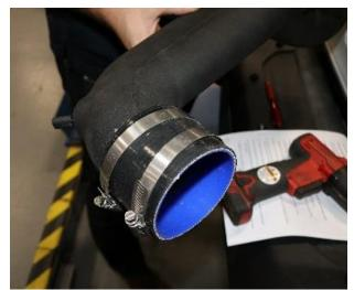
**7.** Locate the CORSA air duct, Ø3.25" straight sleeve, and two remaining #56 clamps. Install straight sleeve and one #56 clamp onto air duct and snug clamp to hold straight sleeve in place. Place the other clamp onto straight sleeve.
