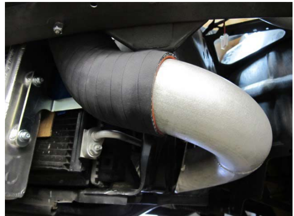
Fig. 6-w: Loosely install discharge tube 'D'
