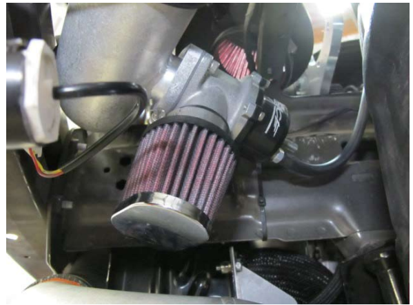
Fig. 7-k: Attach vacuum hose to bypass valve
