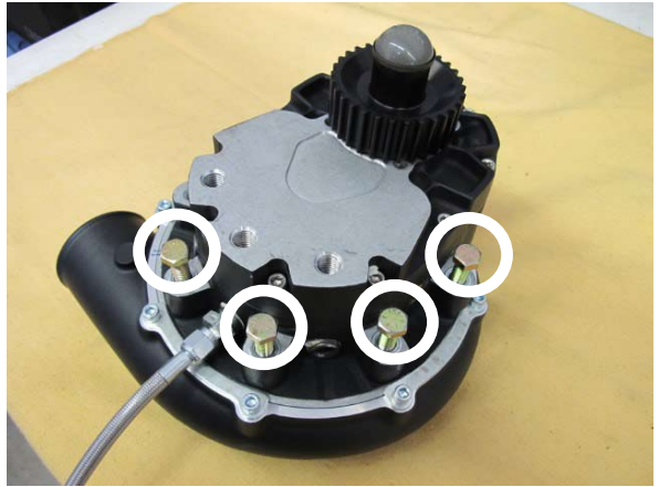
Fig. 7-b: Lubricate supercharger mounting boss threads
