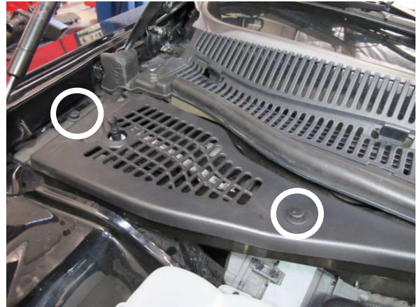
Fig. 1-d: Remove two plastic fasteners
