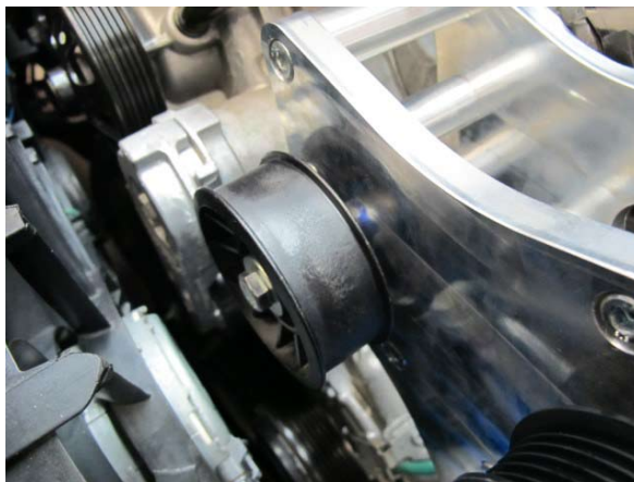
Fig. 5-h: Reinstall serpentine belt idler pulley
