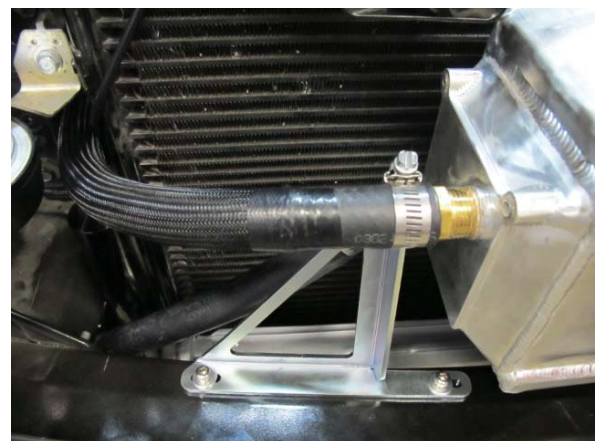
Fig. 8-u: Attach 3/4" coolant hose to air/water cooler
