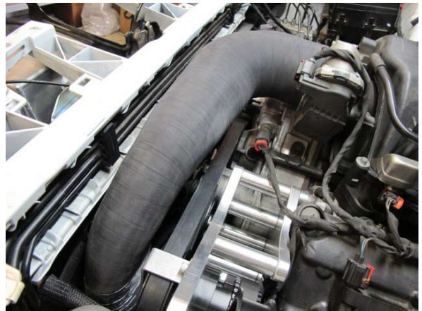
Fig. 6-z: Install discharge sleeve 'E' and reconnect IAT sensor
