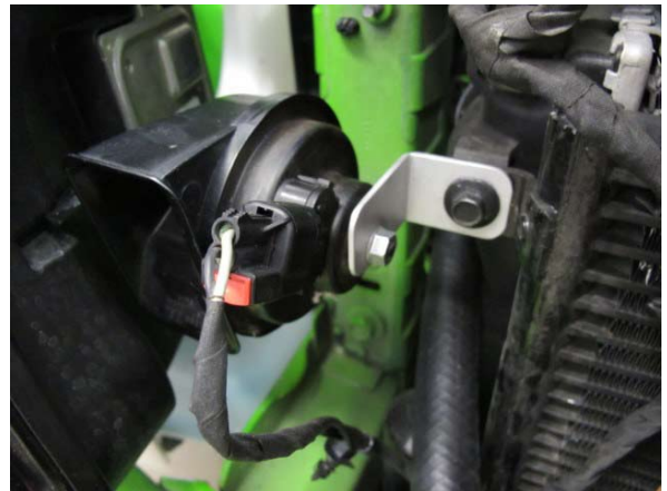
Fig. 6-k: Relocate driver side horn to upper radiator
