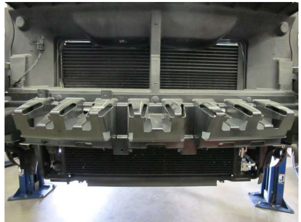
Fig. 2-k: Remove plastic bumper guard
