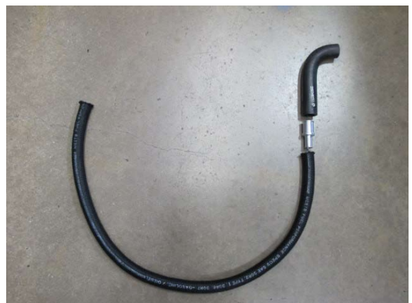
Fig. 7-f: Breather hose assembly
