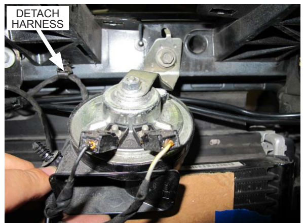
Fig. 6-i: Remove driver side horn
