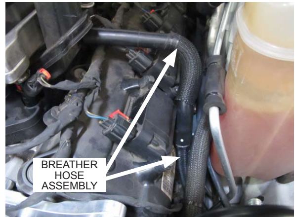
Fig. 7-g: Install breather hose assembly
