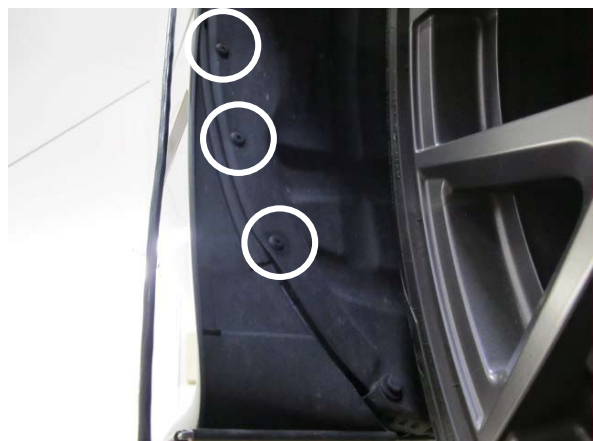
Fig. 2-c: Drill through and remove plastic rivets
