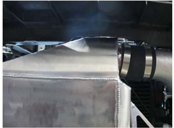
Fig. 9-e: Modified radiator shroud to air/water cooler clearance
