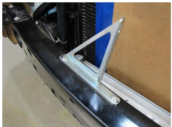
Fig. 6-o: Loosely install passenger side air/water cooler support bracket
