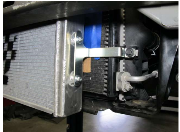
Fig. 6-h: Install driver side of heat exchanger assembly
