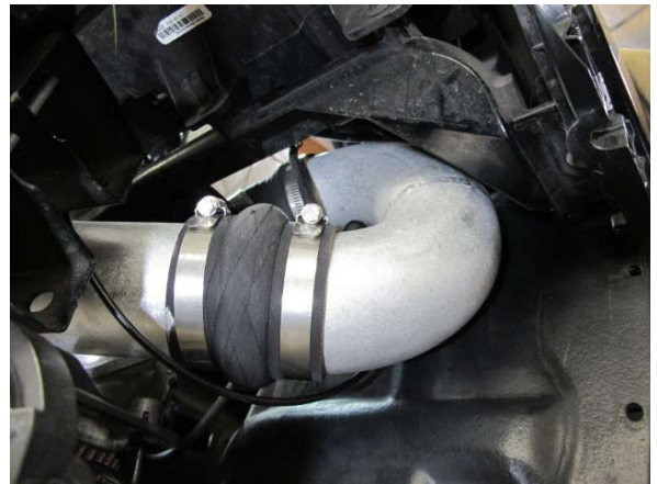
Fig. 6-ac: Loosely install discharge tube 'A' to discharge tube 'B'
