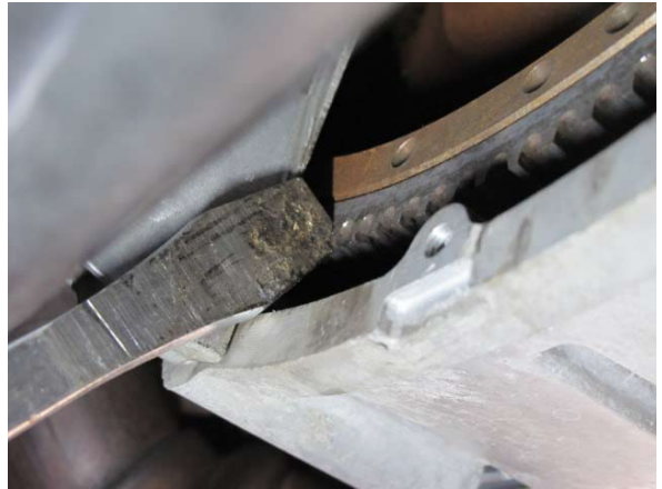
Fig. 3-g: Lock engine in position
