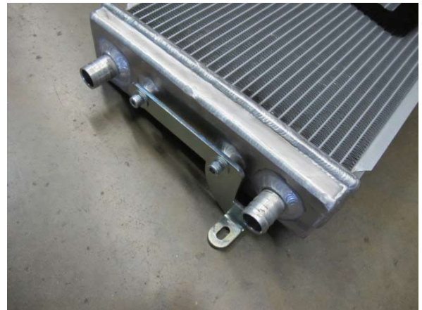
Fig. 6-e: Install passenger side heat exchanger bracket
