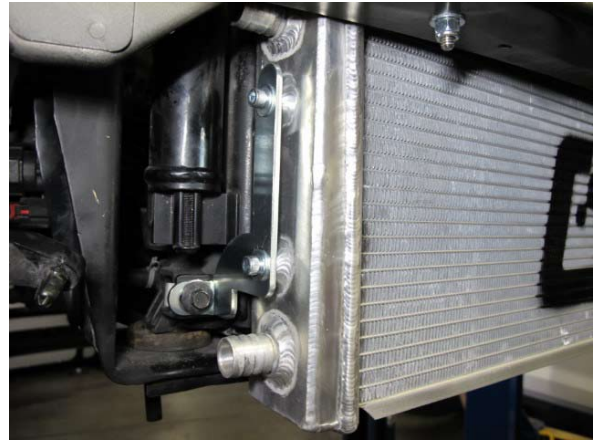
Fig. 6-g: Install passenger side of heat exchanger assembly
