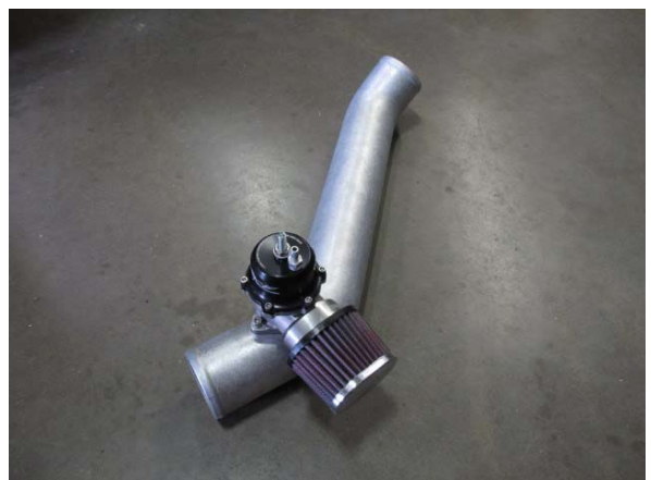
Fig. 6-aa: Install bypass valve to discharge tube 'B'
