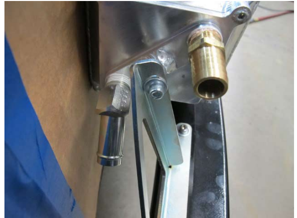
Fig. 6-p: Temporarily secure passenger side of air/water cooler
