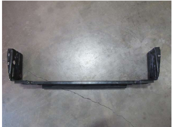
Fig. 4-b: Lower radiator support
