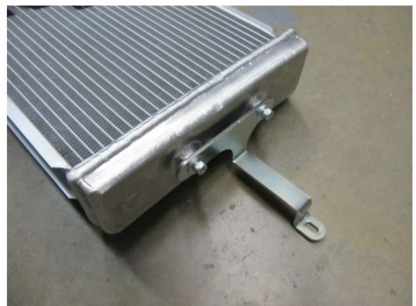
Fig. 6-f: Install driver side heat exchanger bracket
