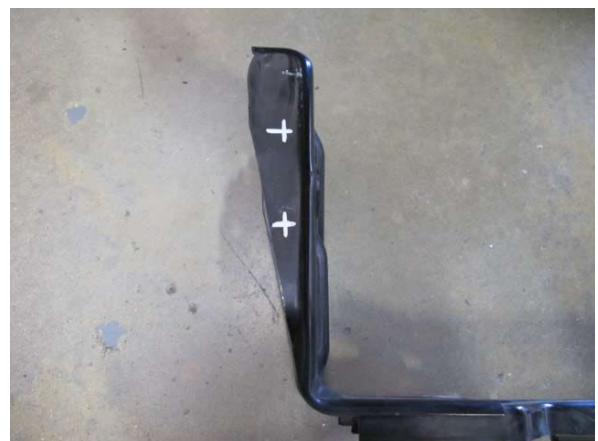
Fig. 4-f: Drill holes on driver side rear edge of lower radiator support
