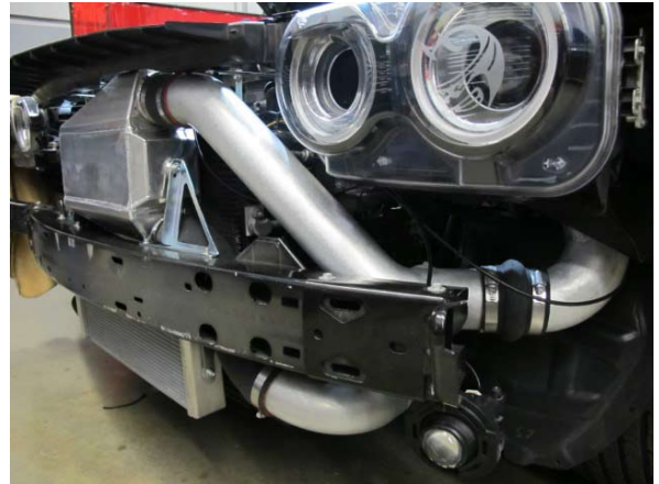
Fig. 6-ab: Install discharge tube 'B'
