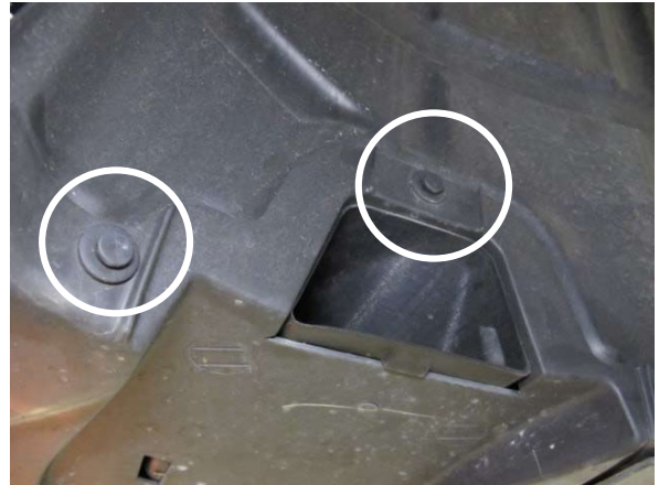
Fig. 2-d: Remove two plastic fasteners
