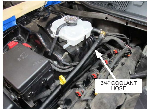
Fig. 8-s: Route 3/4" coolant hose towards air/water cooler
