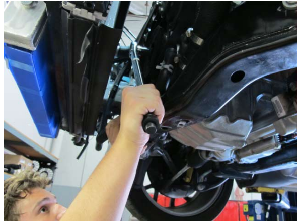
Fig. 3-h: Torque crank bolt
