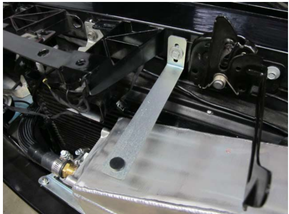
Fig. 9-a: 1.00" width radiator shroud bracket with rubber mount
