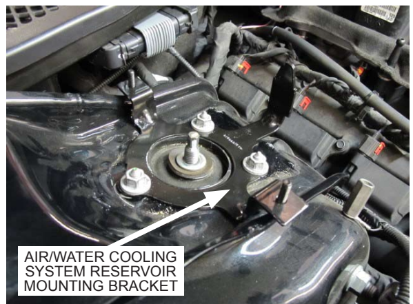
Fig. 8-l: Install air/water cooler system reservoir mount
