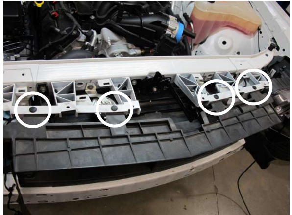
Fig. 2-m: Remove radiator shroud and fasteners
