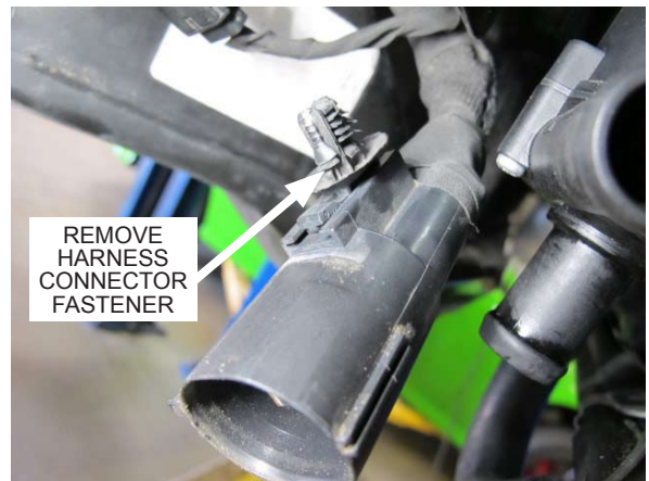
Fig. 8-e: Remove plastic harness connector fastener
