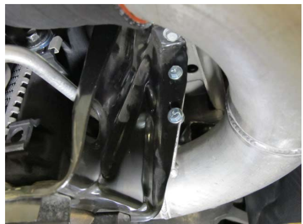
Fig. 6-x: Secure discharge tube 'D' to lower radiator support
