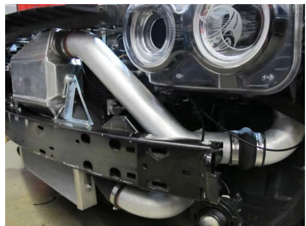
Fig. 7-i: Secure discharge tubes and discharge sleeves
