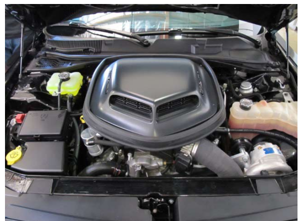
Fig. 10-f: Reinstall shaker base and shaker scoop
