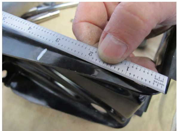
Fig. 4-c: Measure 3.25" from bottom edge
