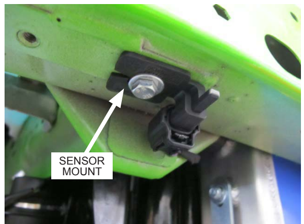
Fig. 6-ad: Reinstall ambient air temperature sensor as shown
