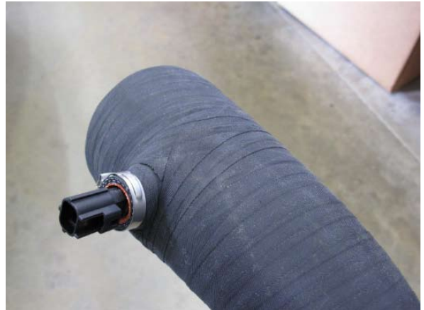
Fig. 6-y: Install IAT sensor to molded boss on discharge sleeve 'E'
