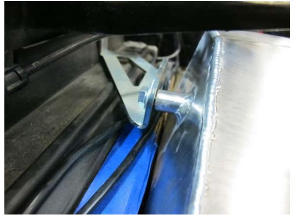
Fig. 6-q: Temporarily secure top side of air/water cooler
