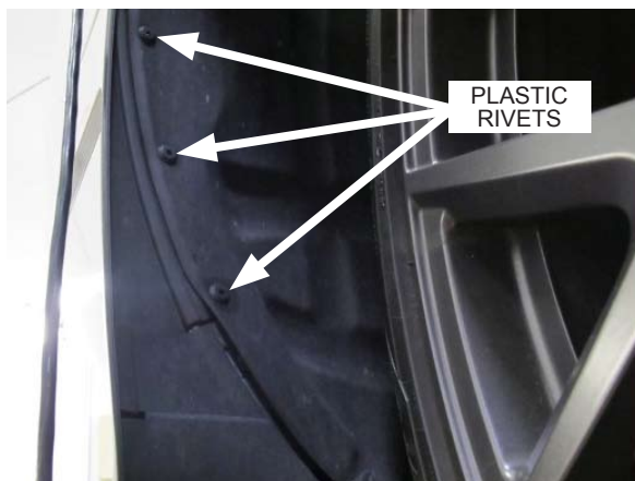
Fig. 10-c: Resecure using provided plastic rivets
