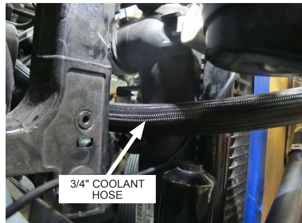
Fig. 8-t: Pass 3/4" coolant hose between radiator and core support
