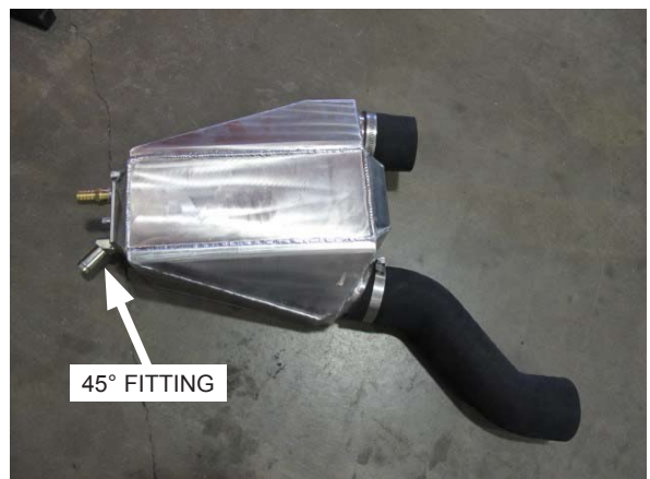
Fig. 6-u: Install silicone sleeves to air/water cooler as shown
