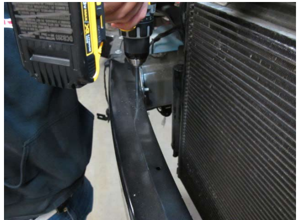
Fig. 6-n: Drill through two holes on front bumper support
