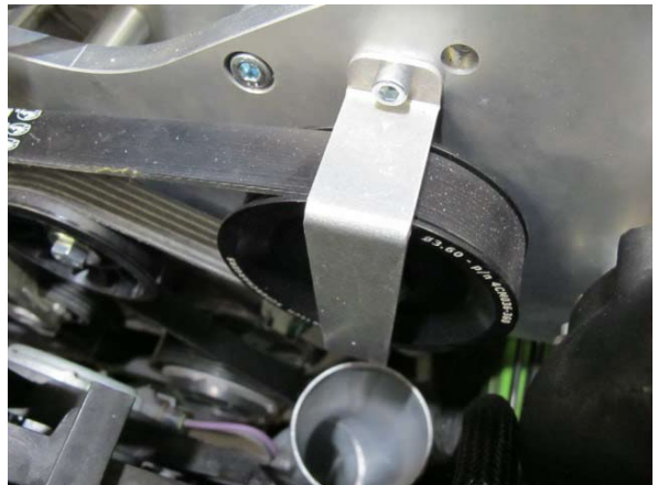
Fig. 5-j: Reinstall pulley guard
