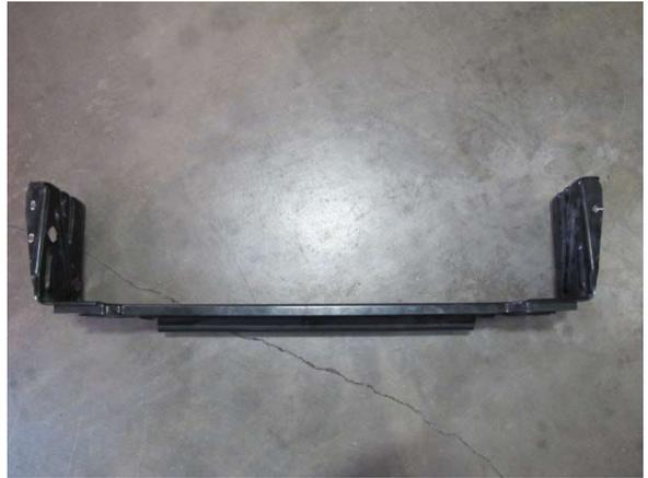
Fig. 4-b: Lower radiator support
