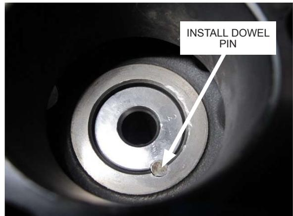
Fig. 3-e: Install dowel pin
