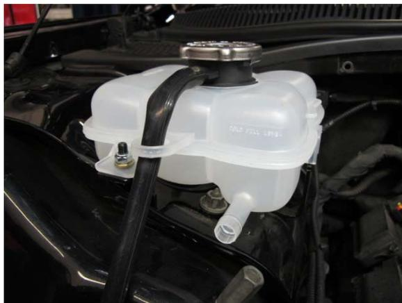
Fig. 8-m: Install air/water cooler system reservoir to mount
