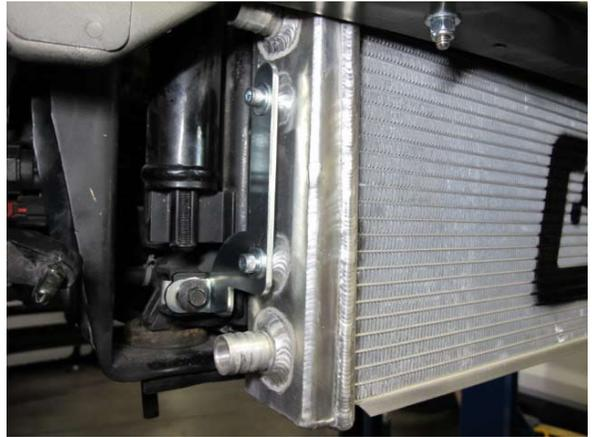
Fig. 6-h: Install passenger side of heat exchanger assembly
