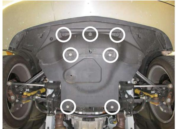
Fig. 2-d: Remove engine service panel fasteners
