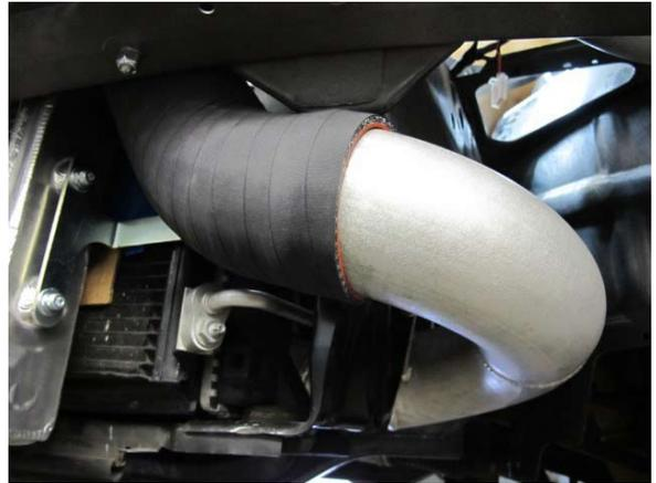
Fig. 6-y: Loosely install discharge tube 'D'
