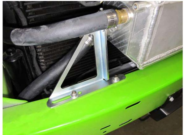
Fig. 6-w: Loosely install passenger side air/water cooler support bracket
