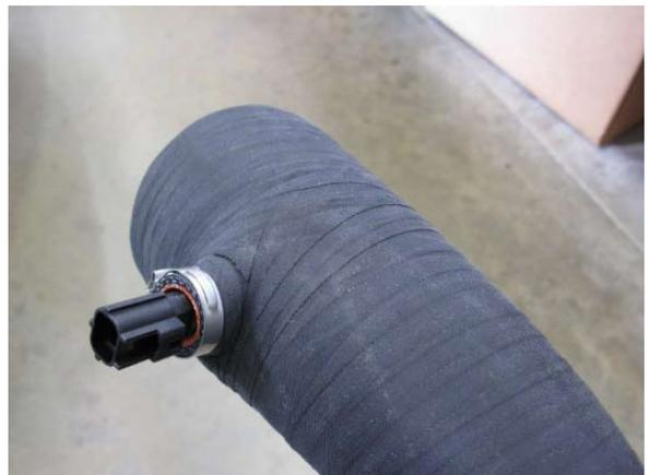
Fig. 6-aa: Install IAT sensor to molded boss on discharge sleeve 'E'
