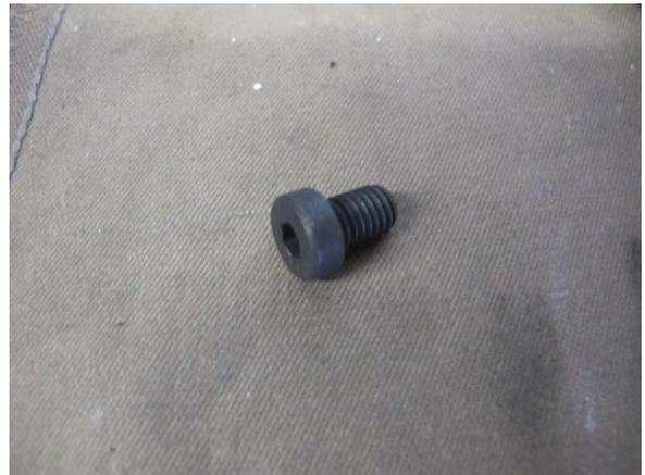
Fig. 8-h: Shorter front bumper support screw
