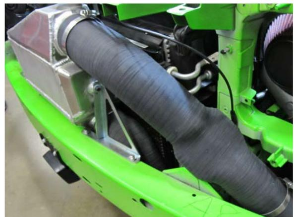
Fig. 6-ad: Install discharge sleeve 'B'
