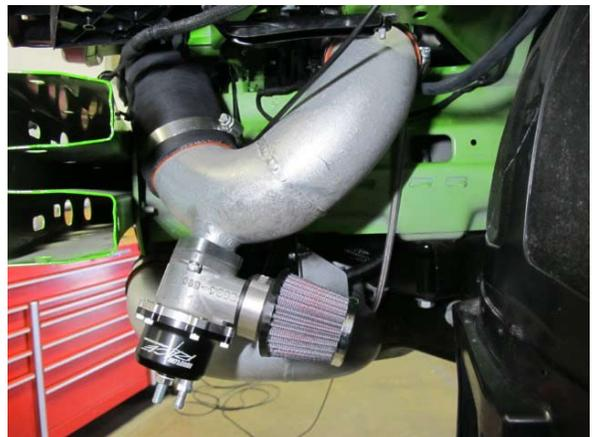
Fig. 6-ag: Loosely install discharge tube 'A' to discharge tube 'B'
