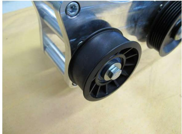
Fig. 5-b: Remove serpentine belt idler pulley
