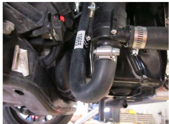
Fig. 8-x: Install coolant hose to electric water pump inlet
