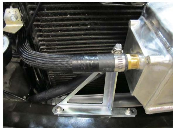
Fig. 8-u: Attach 3/4" coolant hose to air/water cooler
