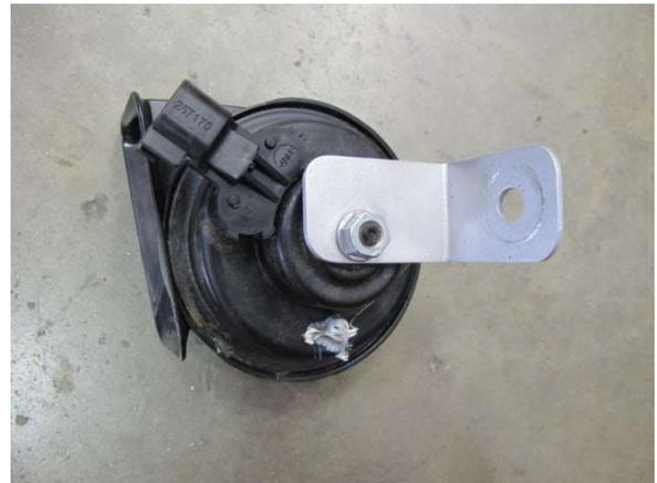
Fig. 6-k: New horn bracket
