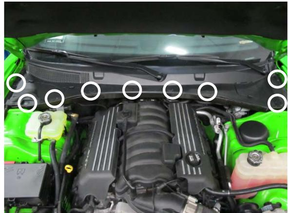
Fig. 1-b: Remove plastic fasteners
