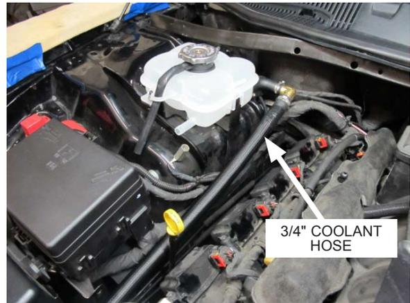
Fig. 8-s: Route 3/4" coolant hose towards air/water cooler
