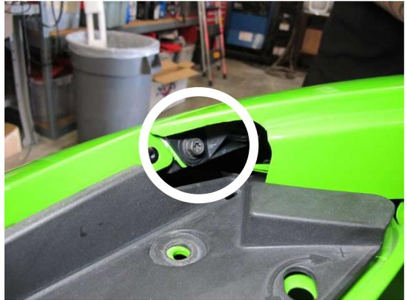
Fig. 2-g: Remove each upper front bumper cover screw
