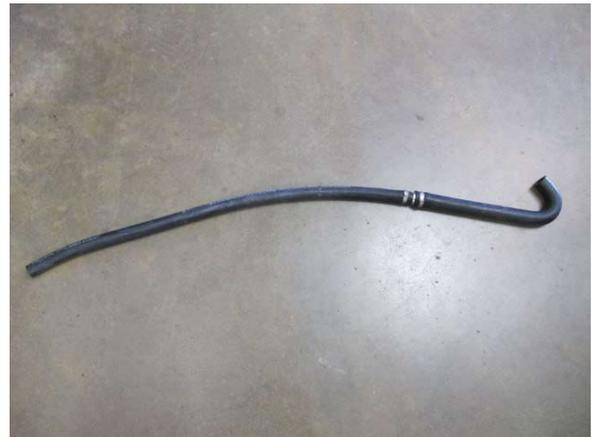
Fig. 8-w: 3/4" x 150° to 1/2" coolant hose assembly
