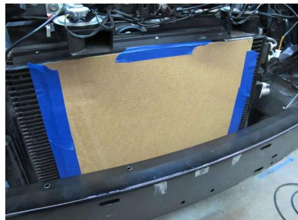
Fig. 6-c: Cover A/C condenser with cardboard
