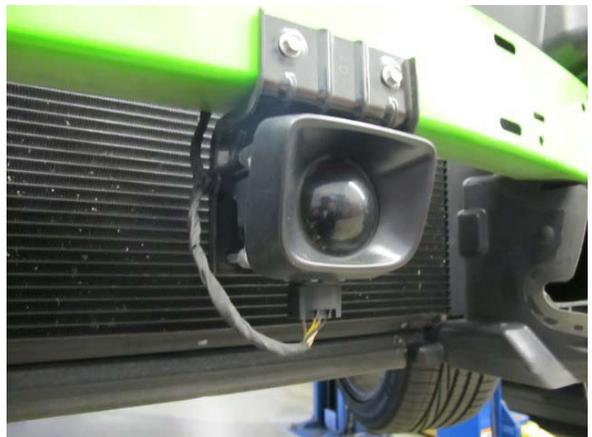
Fig. 2-i: Disconnect adaptive cruise control sensor
