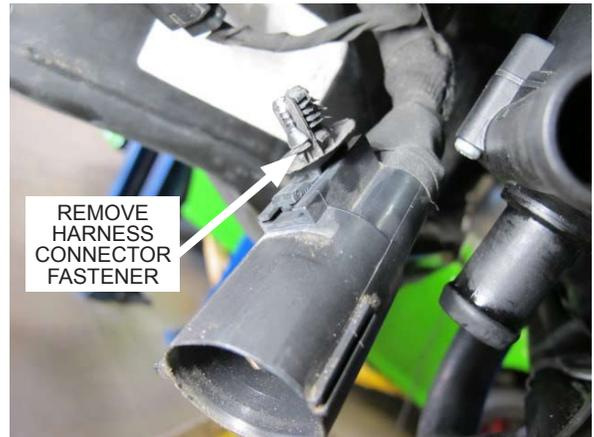
Fig. 8-e: Remove plastic harness connector fastener
