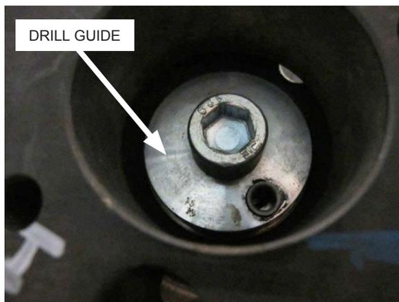
Fig. 3-b: Install drill guide
