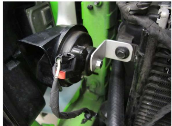
Fig. 6-l: Relocate driver side horn to upper radiator
