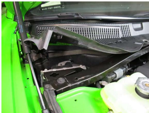
Fig. 1-d: Lift up passenger side of windshield cowl
