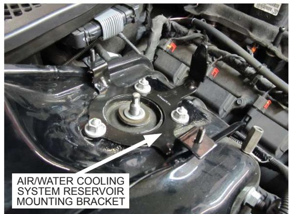
Fig. 8-l: Install air/water cooler system reservoir mount
