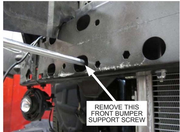
Fig. 8-g: Remove front bumper support screw
