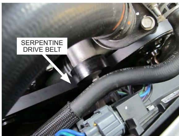
Fig. 5-i: Slide serpentine belt under OEM passenger side smooth idler pulley
