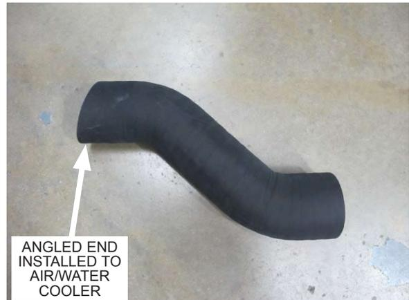
Fig. 6-s: Discharge sleeve 'C'
