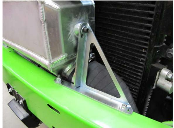
Fig. 6-v: Loosely install driver side air/water cooler support bracket
