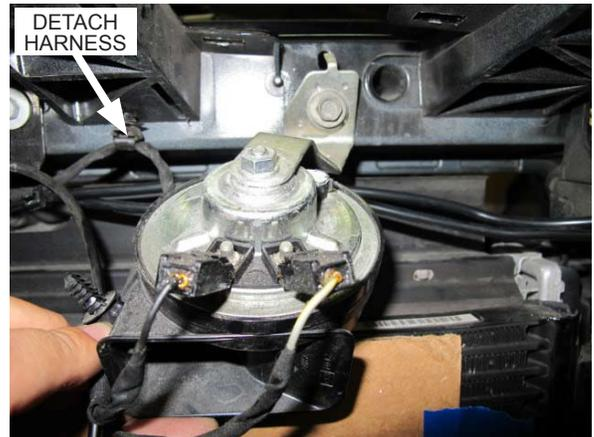
Fig. 6-j: Remove driver side horn
