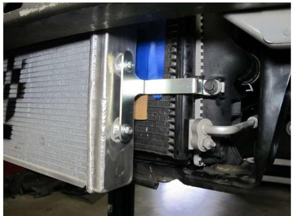
Fig. 6-i: Install driver side of heat exchanger assembly
