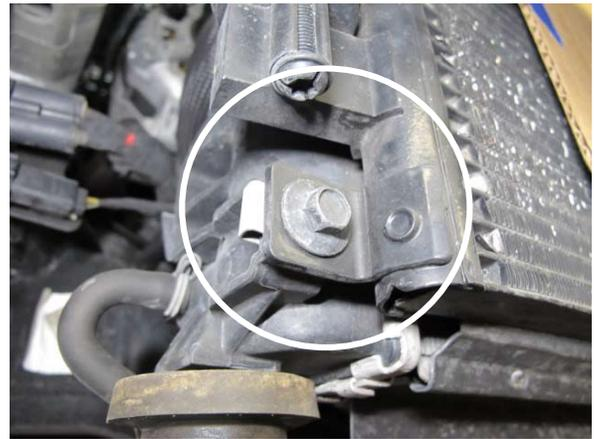
Fig. 6-e: Remove screw
