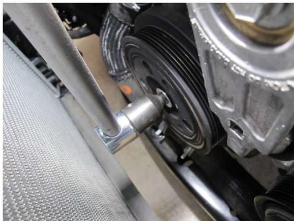
Fig. 3-a: Remove crankshaft damper bolt
