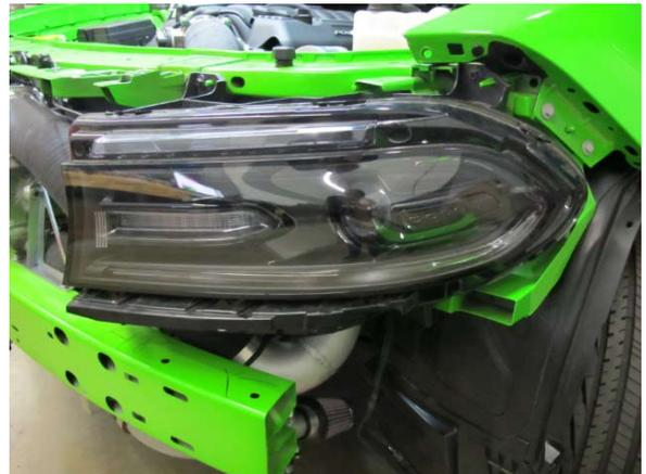
Fig. 6-ac: Remove driver side headlight
