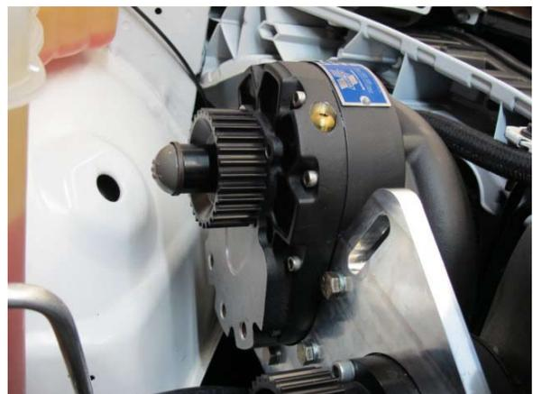
Fig. 7-c: Install supercharger to supercharger mounting bracket assembly
