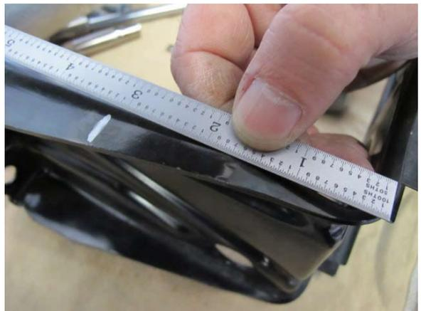
Fig. 4-c: Measure 3.25" from bottom edge
