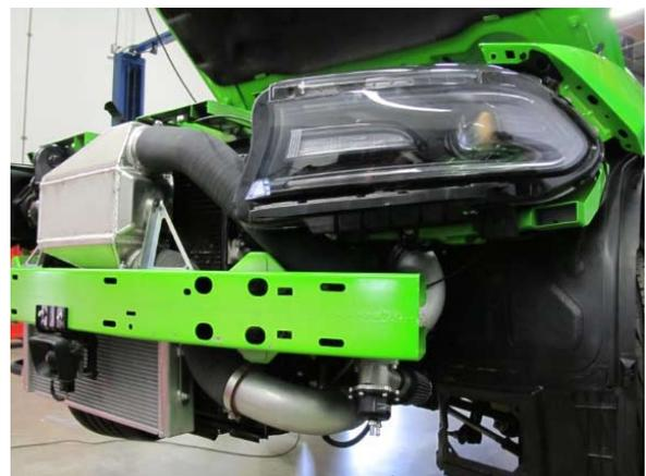
Fig. 7-i: Secure discharge tubes and discharge sleeves
