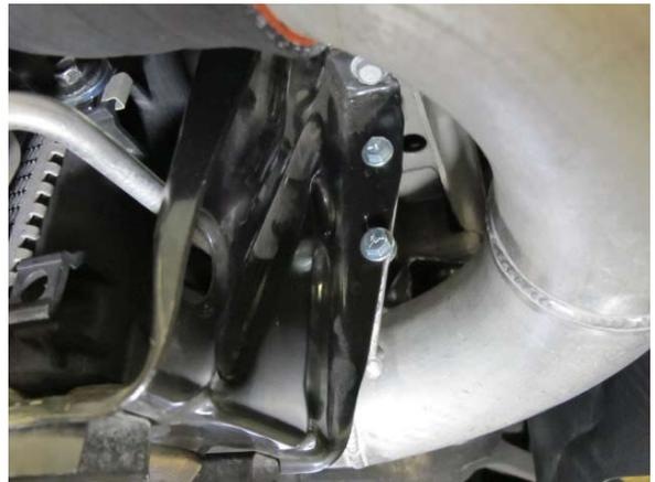
Fig. 6-z: Secure discharge tube 'D' to lower radiator support
