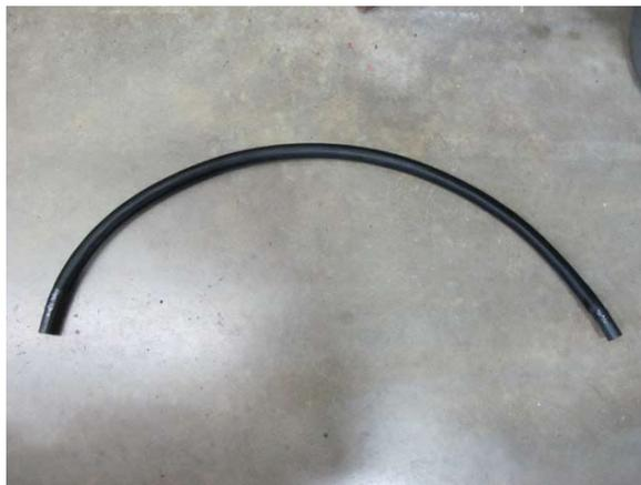
Fig. 8-n: 44" length of the 3/4" coolant hose
