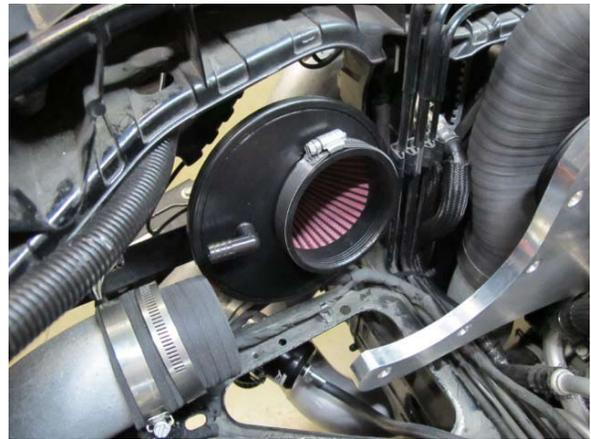
Fig. 7-a: Place air filter into position and install silicone sleeve to discharge tube 'A'
