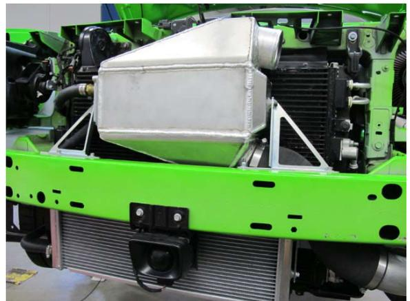
Fig. 6-x: Install air/water cooler
