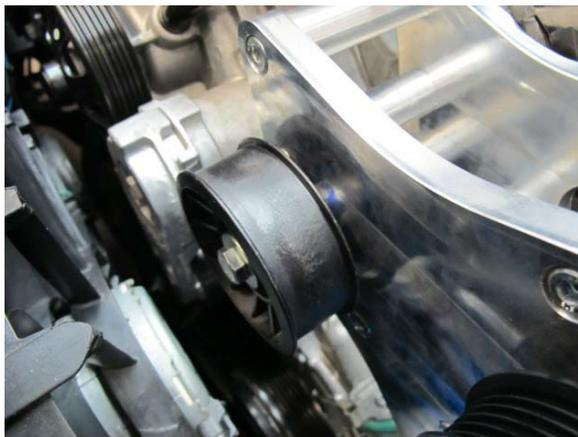
Fig. 5-h: Reinstall serpentine belt idler pulley
