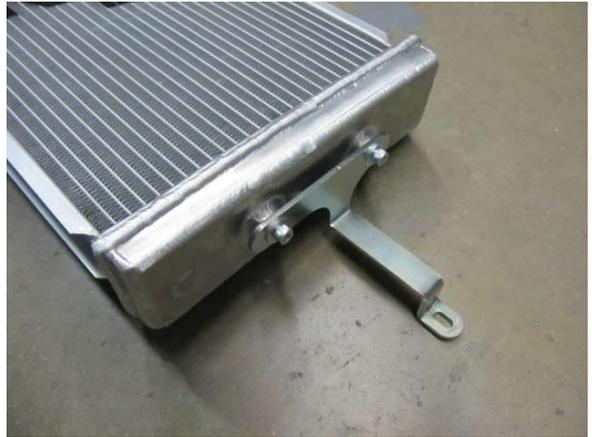
Fig. 6-g: Install driver side heat exchanger bracket
