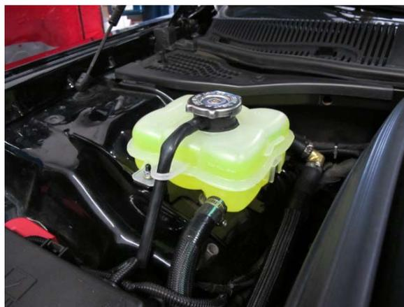
Fig. 8-z: Fill air/water cooling system with 50/50 water/coolant mix
