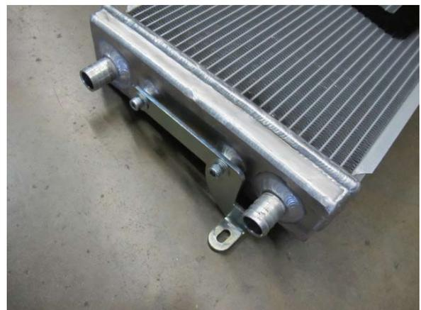
Fig. 6-f: Install passenger side heat exchanger bracket
