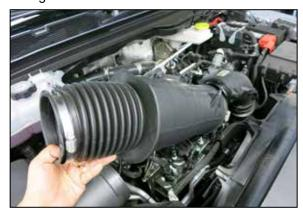
7. Disconnect the intake tube from the air-filter housing and then remove it from the vehicle.
