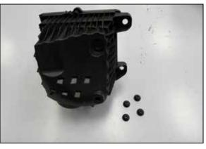
9. Remove the four mounting grommets from the factory air filter housing.
