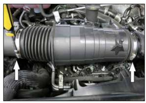
5. Loosen the hose clamps that secure intake tube to the air filter housing and intake plenum.
