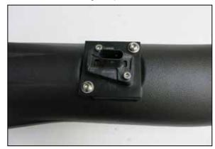
15. Remove the mass air sensor from the factory housing and install it into the adapter installed onto the K&N intake tube.
