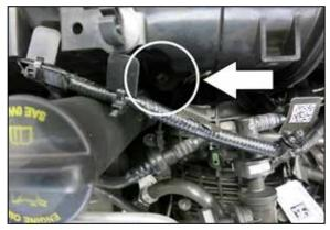
6. Remove the bolt that secures the intake tube to the engine.
