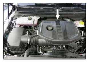
2. Remove the bolt that secures the center of the engine cover then lift the cover up and remove it from the engine.
