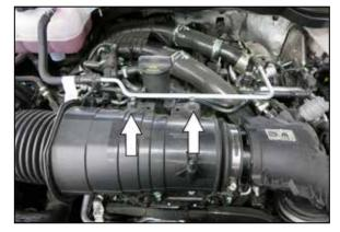
3. Disconnect the coolant by-pass line from the factory intake tube.
