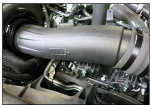
17. Install the K&N intake tube assembly into the air filter and then into the coupler, the coupler will need to flexed around the tube. Align the tube for
