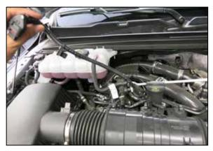
4. Disconnect the mass air sensor electrical connection and then unhook the harness from the intake tube.
