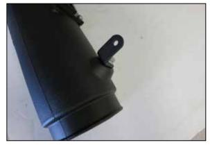
14. Install the provided mounting bracket onto the K&N intake tube using the provided hardware.
