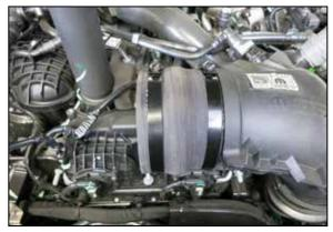
16. Install the provided hump coupler onto the intake plenum with the provided hose clamp. Tighten clamps using 5/16" socket or nut driver. **Note: Do not over tighten clamps.**
