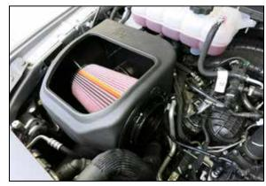
12. Install the K&N air filter into the air filter housing.
