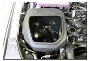
10. Install the four-factory air filter housing mounting grommets into the K&N air filter housing and then install the K&N housing into the vehicle so the mounting pins protrude through the grommets.
