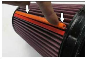
11. Attach the filter clips to the pleats on the air filter align and push down. Passenger side filters, place orange clip on top and red on bottom.
