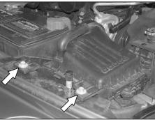
Remove the two airbox retaining bolts.
