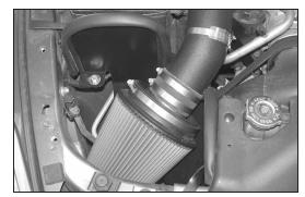
29. Install the K&N® air filter assembly onto the K&N® intake tube and secure with the provided hose clamp.
