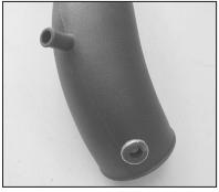
18. Install the provided grommet into the K&N® intake tube as shown.
