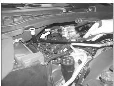
7a. On 2006 and later vehicles, disconnect the crankcase vent tube from the rear of the intake manifold.
