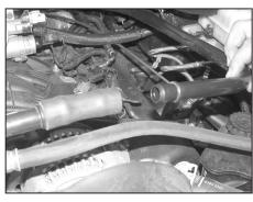
2. On 2005 and earlier vehicles. Disconnect the crankcase vent tube from the vent hose junction above the alternator.
