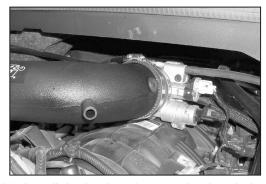
21. Install the intake tube onto the throttle body with the provided hose clamp.
