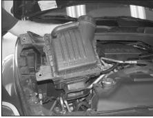
5. Pull up firmly to dislodge the airbox from mounting grommet, and remove the airbox from the
