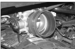
16. Install the silicone hose (08051) onto the throttle body and secure with the provided hardware.
