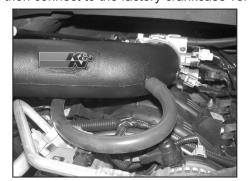
24a. On 2006 and later vehicles connect the crankcase vent hose installed in step #7c to the K&N® intake tube as shown.
