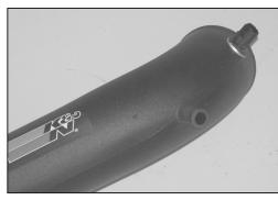
20. Install the air temp sensor into the  $K\&N^{\mbox{\scriptsize 6}}$  intake tube as shown.
