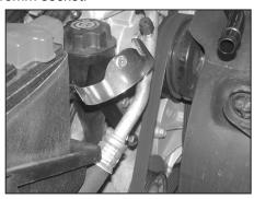
10. Install the tube bracket assembly onto the engine using the provided hardware, threading the bolt into the vacated hole by the bolt removed in step #9.
