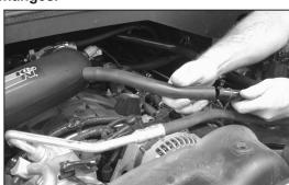
24. On 2005 and earlier vehicles connect the provided silicone hose to the K&N® intake tube, then connect to the factory crankcase vent tube.
