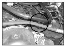
26. On 2006 and earlier vehicles install the crankcase vent tube mounting clip onto the a/c line and crankcase vent tube as shown.
