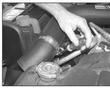
22. Using the provided hose clamp, secure the  $K\&N^{@}$  intake tube to the saddle bracket assembly as shown.
