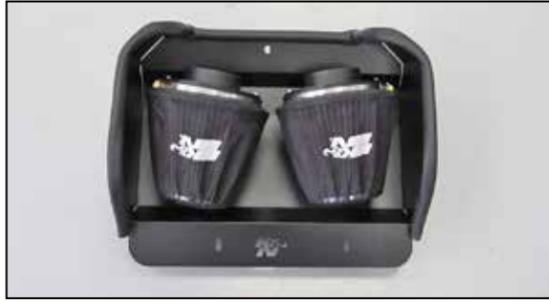
12. Install the K&N® air filter assemblies onto the filter adapters and secure with the provided hose clamps.
