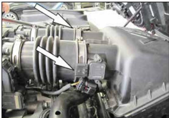
2. Unplug the two mass air sensor electrical connections.
