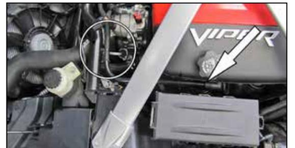
6. Unhook the crank case vent tube retaining clip from the frame cross member. Remove the crank case vent tube from the 90° fitting at the valve cover and then remove the tube from the vehicle.
