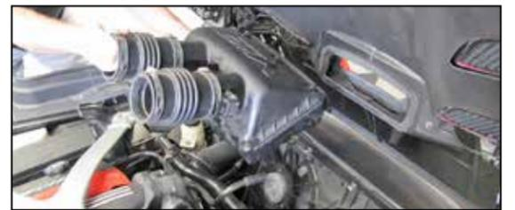
5. Remove the two thumb screws which secure the front of the factory air box to the core support, lift up the air box to unhook it from the mounting grommet. Disconnect the intake hoses from the throttle bodies and then remove the air box assembly from the vehicle.
