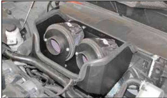
15. Install the heat shield assembly into the vehicle so that the inserted nut installs into the factory air box mounting grommet location. Secure the heat shield with the hardware provided to the factory air box mounting locations.
