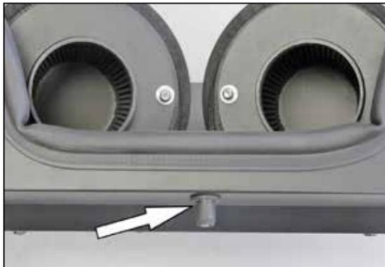
13. Install the provided inserted nut onto the heat shield as shown.
