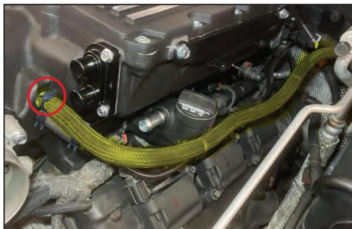
143. Select the coolant reservoir mounting bracket PN 65-26-61-029 and (2) M8X1.25X16 fasteners PN 71-08-12-016. Install the bracket to the LH side of the supercharger using the 2 fasteners as shown. **Torque the fasteners to 11 ft-lbs.**
