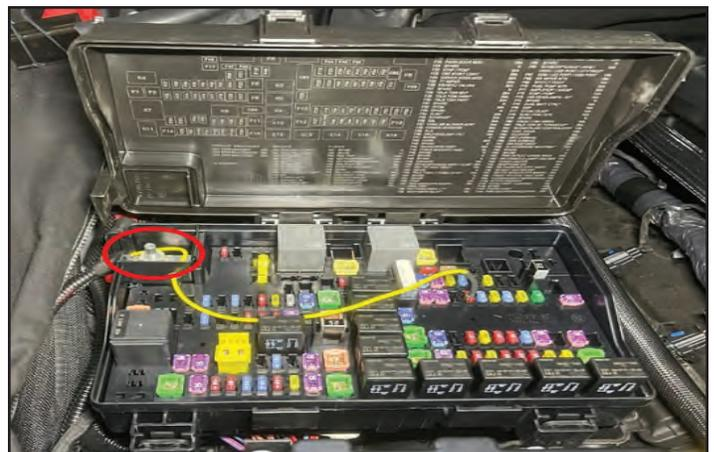
97. Select the relay harness assembly from the kit. Install the RED wire with the ring terminal on the end over the B+ terminal inside the fuse box then secure it with the original nut. Notch the fuse box cover as necessary for clearance to the red wire.
