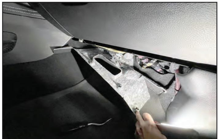
21. Re-secure the close out panel by pushing the (3) fir tree connectors back into place in the locations shown (Durango shown, Grand Cherokee similar).
