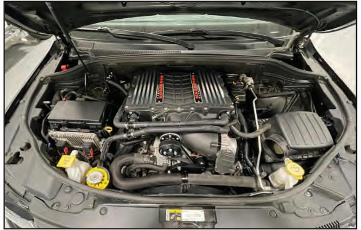
196. Test drive your vehicle for a while taking care to not get into boost immediately. **Do not perform any wide open throttle tests at this time.** Pay close attention to the sounds of your engine, if you notice detonation (pinging) back off immediately and contact your installation facility. The supercharger does have a whining sound while under boost. When you are through with the initial test drive check again for any leaks, and top off with coolant if necessary.
