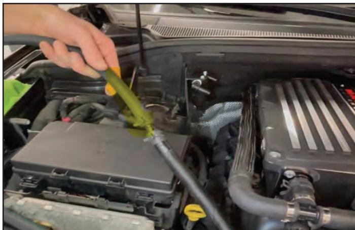
151. Route the length of bulk hose toward the front port on the oil separator, cut it to the appropriate length and install it, ensuring it is fully seated. A clamp is not required. Zip tie the hose against the wiring harness to secure it..
