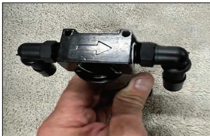
145. Mount the oil separator to the supplied bracket (arrow faces toward the front of the vehicle) using 2 self-tapping fasteners PN **74-74-08-038** then install the bracket onto the (2) factory studs on the top of the RH shock tower at the location shown. Secure it using (2) M6 nuts from the kit.
