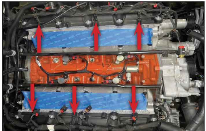
132. Carefully cut and remove the zip tied connections from the harness at all (6) locations.
