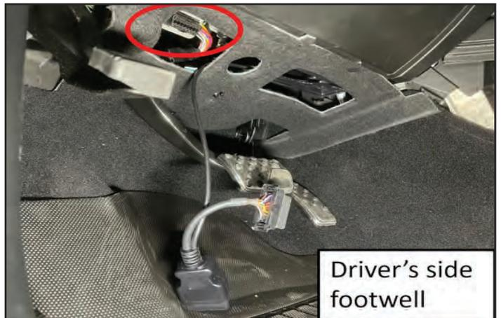
16. Plug the OBD connector into the factory port, ensuring it is fully seated.
