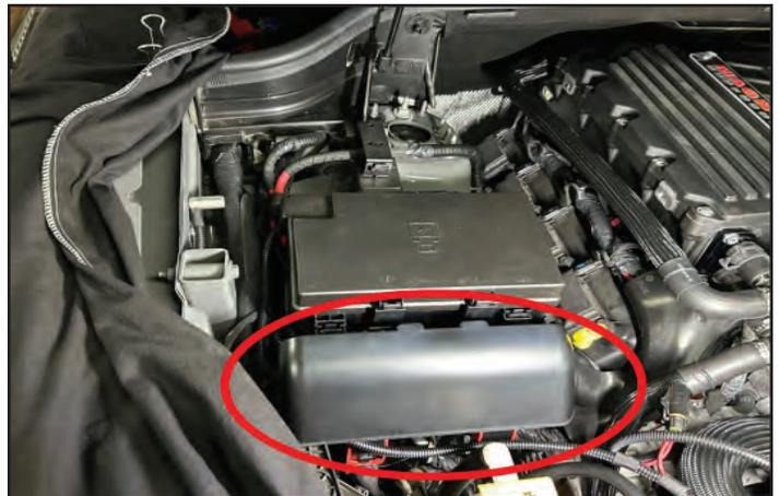
7. Take the PCM to a work bench and remove the (2) nuts that secure it to the bracket. Carefully package the PCM and ship it out to be updated as per the instruction.
