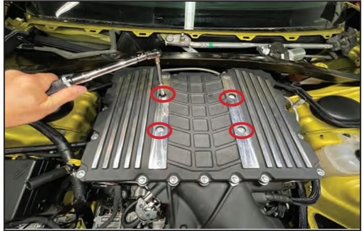
138. Select the charge air cooler turrets. Apply Lubriplate to the O-rings as shown below then re-install them to the appropriate sides of the supercharger. **Re-install the original turret fasteners, run them down then final torque them to 106 in-lbs.**
