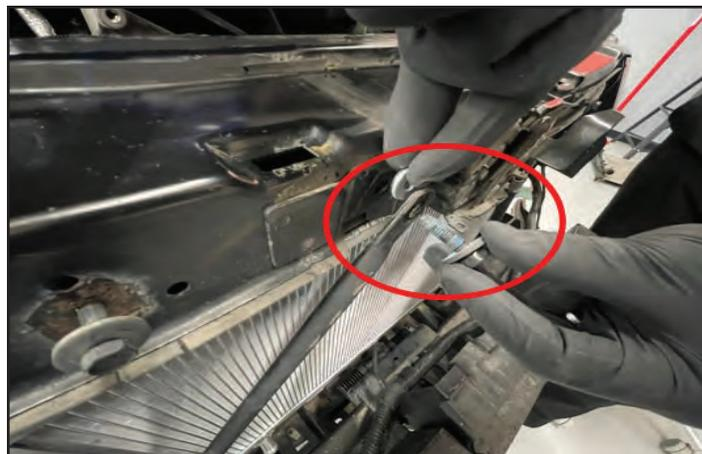
87. Re-install the horns into their factory locations and secure them using the factory bolts. Ensure the horns and horn harnesses do not touch the LTR after installation. The horn brackets can be bent slightly as required.
