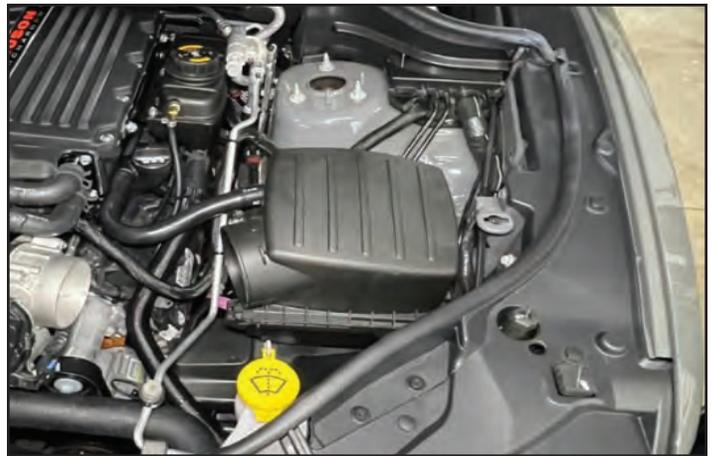
171. Connect the rubber hose from the airbox lid to the oil fill adaptor as shown. Secure both sides of the hose with a constant tension clamp at the circled areas.
