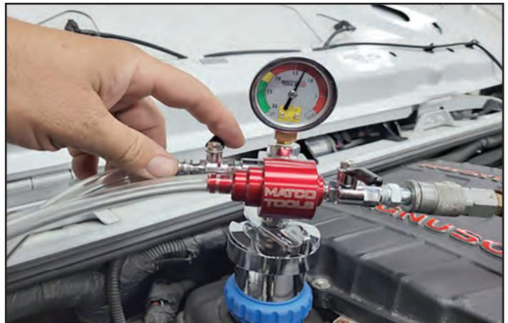
188. **Refill BOTH the intercooler AND engine coolant systems.** Slowly open the fill valve and purge all the air out of the fill hose to avoid any air being introduced during the fill process, and once the coolant gets to the valve close it.
