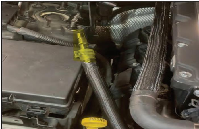
150. Select the ½” I.D. bulk hose from the kit. Install it onto the mender and secure it with another 21mm constant tension clamp.
