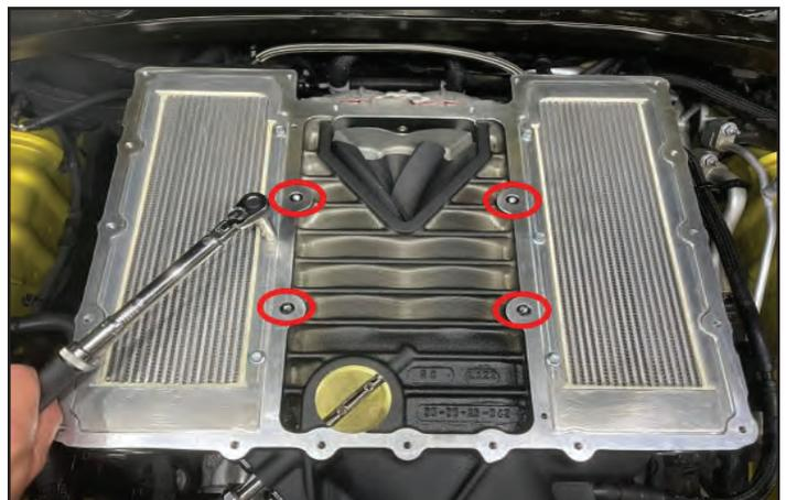
137. Re-install the supercharger lid onto the housing. Re-install all the lid fasteners. Make sure to remove the Magnuson badges to allow access to the four center bolt (M6x30mm) locations circled in red here. These M6x30mm bolts are located in a supplied bag. Follow the sequence for the lid bolts shown at the back of this manual. Zero torque the fasteners first before applying the final torque. **Final torque the lid fasteners to 106 in-lbs.**
