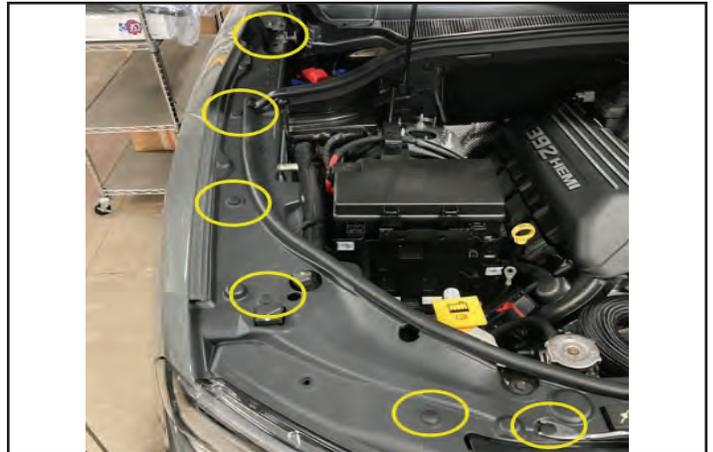
23. Repeat the removal process for the LH side engine bay cover, including the small close out panel by the air filter box. 11 push pins (circled in yellow) secure it to the vehicle on this side. Remove the rubber molding from the front center of the vehicle (red arrows) by pulling up on the fir tree connectors.
