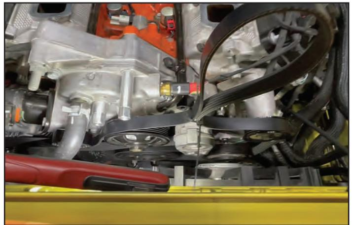
116. Install the bracket sub-assembly onto the front of water pump housing, ensuring the spacers stay on the fasteners. Ensure the belt is routed below the LH stand-off and in between the two idler pulleys as shown. **Torque (3) bracket bolts 18 ft-lbs.**
