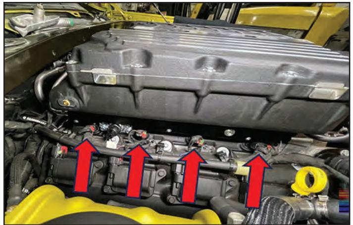
140. Route the factory fuel vapor line toward the left front corner of the supercharger. Remove the 90-degree rubber elbow from the end of the fuel vapor line. **Select the length of 3/8" bulk hose from the kit. Cut a 3" long piece of hose off one end.** Secure the hose to the fuel vapor line using a constant tension clamp from the kit at the red arrow. Install the fuel vapor line onto the lower port on the supercharger inlet as shown with another constant tension clamp at the yellow arrow.
