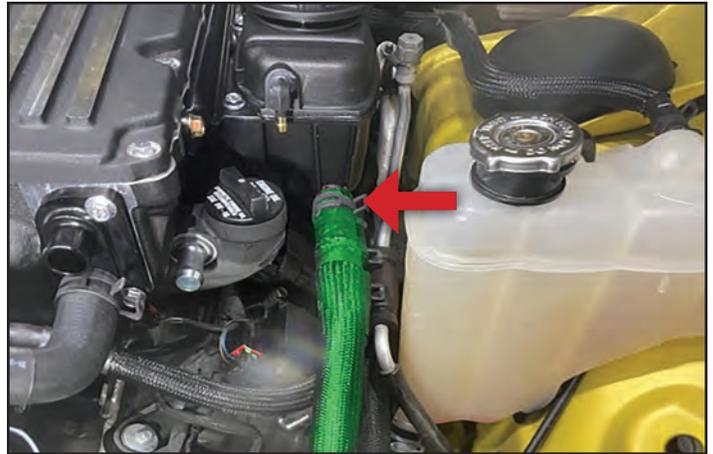
163. Find the 1/4" hose previously installed to the low temp radiator. Route the 1/4" hose along side the 3/4" hose installed in the previous slide. Trim the hose to length as necessary then apply Lubriplate to the hose barb on the reservoir and install the 1/4" hose, securing it with a 1/4" constant tension clamp.
