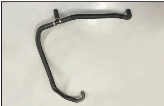
157. Install the 003C hose (highlighted in green) to the **LH and RH LOWER ports on the supercharger**, securing it with 3/4" constant tension clamps from the kit as shown.
