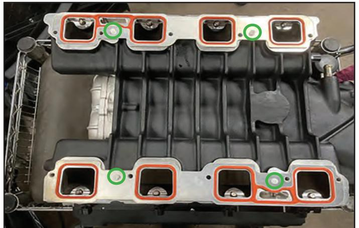
127. If you are installing a boost gauge, there is a spare 1/8" NPT plug on the RH rear corner of the supercharger for this provision.
