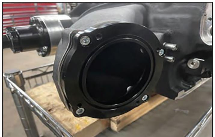
129. Remove the stock throttle body from the factory intake. Harvest the factory throttle body gasket from the intake and install it onto the inlet adaptor on the supercharger.
