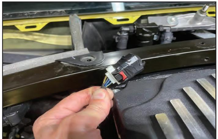
181. Trim the drivers' side plastic close out panel in the location shown to provide clearance for the intercooler pump hose. Re-install the closeout panel then re-attach the ambient air temp sensor. Re-install the passenger side close out panel (not shown but similar to drivers side.)
