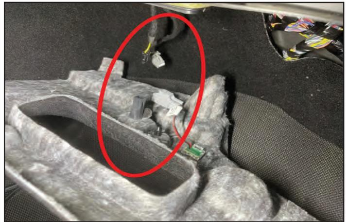
11. Remove the trim panel from the RH side of the center console by gently pulling it away to release it from its' mounting tabs, Set the panel aside (Durango shown, Grand Cherokee similar).
