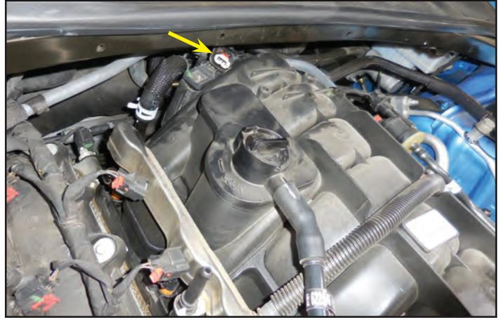
38. Disconnect the EVAP hose from the front of the driver side of the intake manifold behind the throttle body. Pull the EVAP hose clips off from along the manifold.
