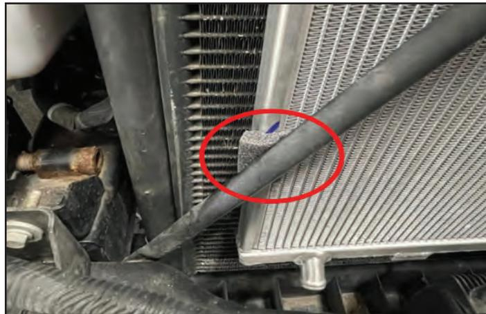
86. Select a thick spacer PN 75-00-08-021 from the kit. Install the spacer behind each pencil brace as shown. Secure the top of the pencil braces using the factory bolts.
