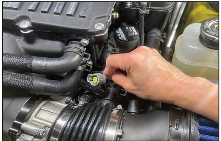
176. Route the jumper harness under the front of the supercharger and over to the sensor located on the RH front corner, under the bypass valve. Plug the harness into the sensor ensuring it locks into place.
