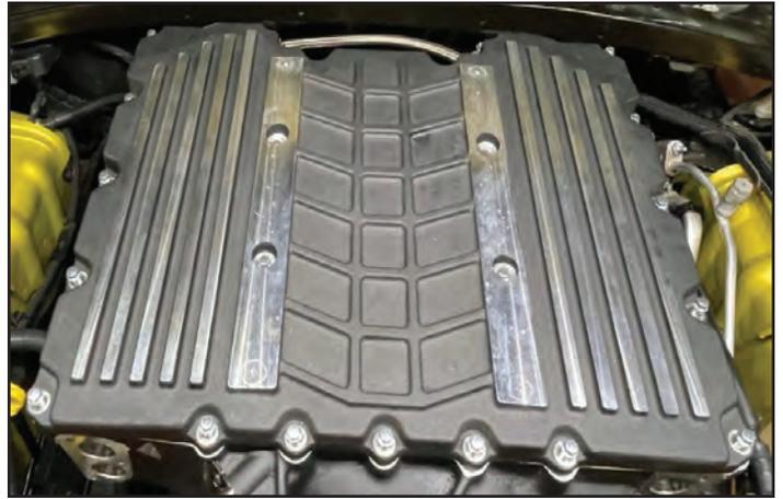
122. Remove (6) internal fasteners securing the CAC's to the base.
