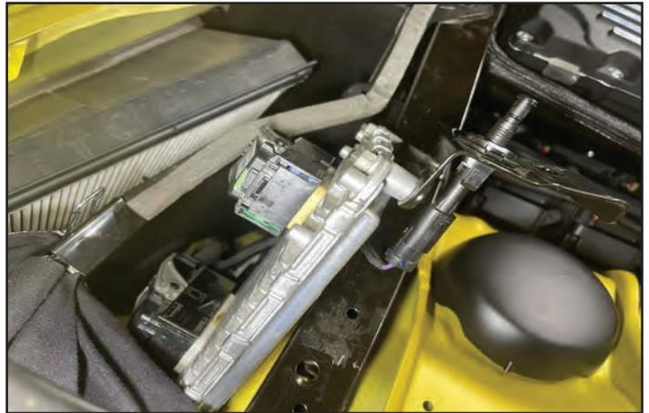
179. Secure the PCM bracket to the cowl using the factory bolt.
