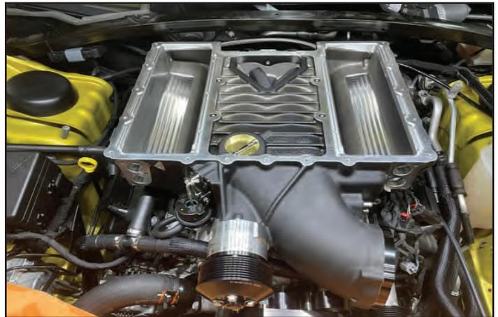
135. **Apply blue Loctite 242** to the (10) M6X1.0X40mm long fasteners and install them into the supercharger mounting locations. Hand-start and zero-torque all fasteners as shown in the diagram at the back of this book. **Pre-torque all 10 fasteners to 53 in-lbs in sequence. Final torque all 10 fasteners to 106 in-lbs in sequence.**
