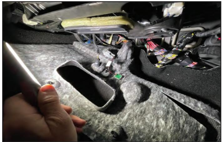
20. Position the close out panel back into place, ensuring it tucks up above the edge of the carpet and under the dash neatly.
