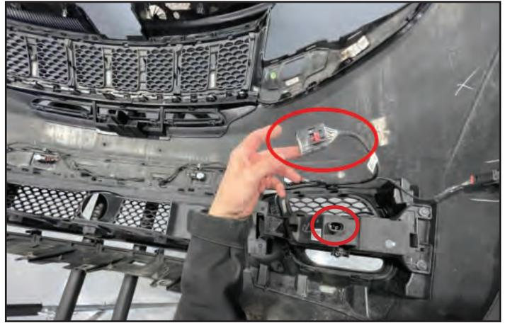
30. Remove the ambient air temp sensor from the drivers' side plastic close out panel then remove the panel from the front of the vehicle. The panel will be modified and re-installed later. Remove the passenger side close out panel (not shown but similar)
