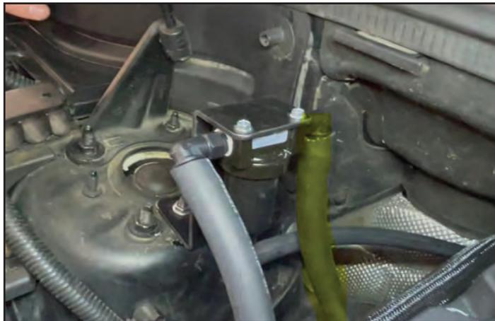
154. Install the OE oil fill cap into the threaded hole at the LH front corner of the supercharger
