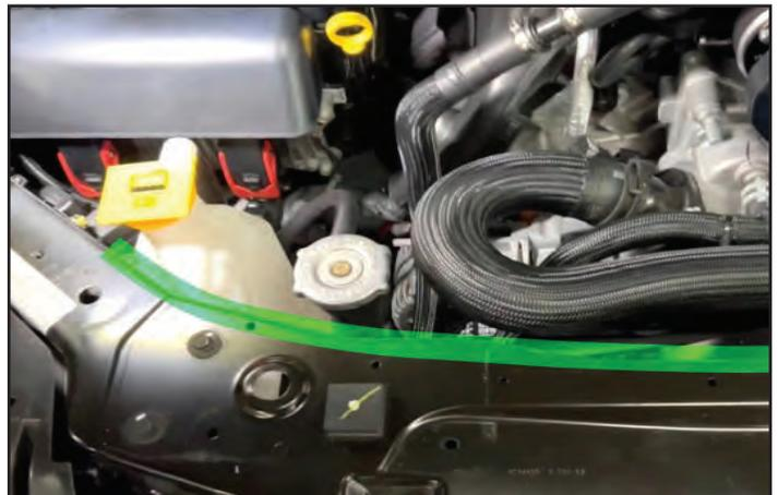
103. Continue routing the harness under the radiator cradle, toward the upper radiator hose connection to the radiator (highlighted in green), then down toward the intercooler pump. Connect the harness to the pump. Bundle any excess wire together by the pump using zip ties. Secure the harness with zip ties along the route as required.
