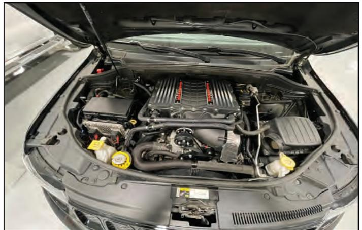
183. Re-fill both coolant systems with Mopar antifreeze PN 68163849AB **Use of a vacuum bleed tool is highly recommended. The intercooler pump will shut down automatically if it detects excessive air in the system. Consult your owners manual and ensure you purchase the correct coolant for your vehicle.**
