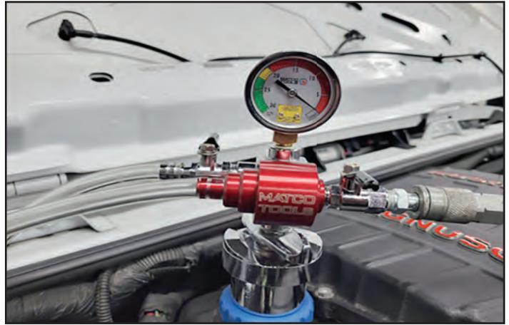
186. **Consult your owner's manual and select the correct coolant for your vehicle. Failure to select a compatible coolant may cause contamination of the coolant system and potentially lead to overheating issues.** Connect the shop air to the tool, and submerge the fill hose into the fill coolant container.
