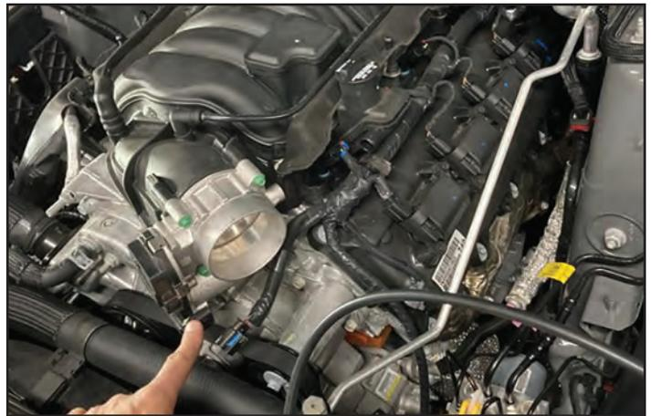
35. Remove LH / RH felt injector covers from the engine. These will not be re-used.
