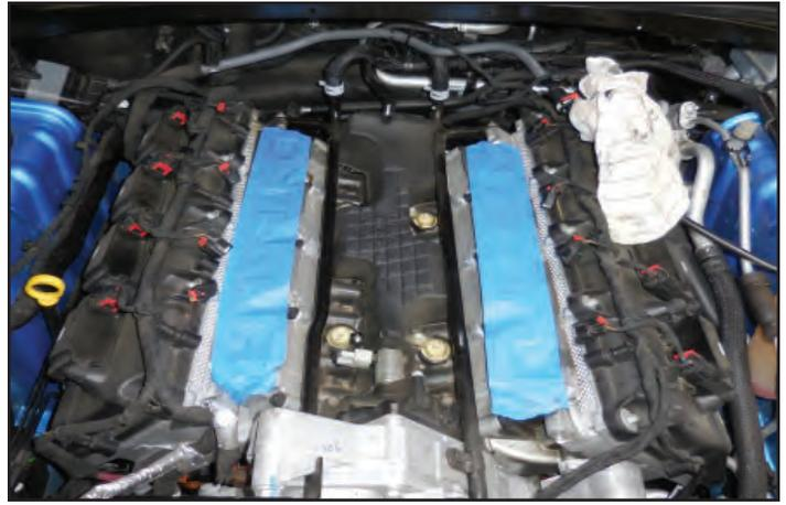
50. Use a 16mm wrench to remove the air box extension support bracket if applicable. Not required on 6.4L vehicles.
