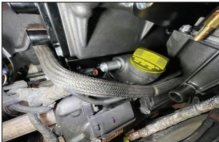
155. **6.4L engines Only:** install MAP sensor jumper harness PN 82-55-80-042 between the new sensor at the LH rear of the supercharger and the factory connector at the RH rear of the engine compartment.
