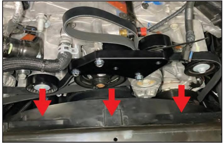
118. Re-fasten the A/C line bracket using the original bolt. **Torque it to 7 ft. lbs.**
