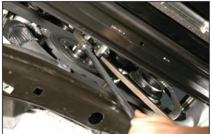
59. Install the crank pin drill guide with the provided bolt and a 22mm wrench. It's convenient to align the two holes for the crank pins in the drill guide horizontally for ease of access. **Torque the temporary bolt holding the drill guide to 40 ft-lbs.**
