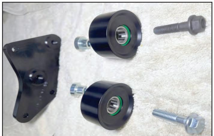
105. Idlers must be installed with the snap ring facing the stand-off on the idler bracket. Clamp the idler and bracket sub-assembly in a vice to secure it then **torque the fasteners to 27 ft-lbs.**
