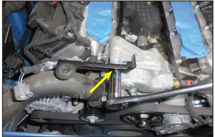
51. To facilitate the hose install, use a long 3/8" drive ratchet to spring the tensioner and remove the OEM fan belt. This belt will not be reused.
