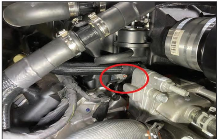
177. Re-install the bracket to the PCM in the orientation shown. Secure the bracket using the (2) factory nuts.
