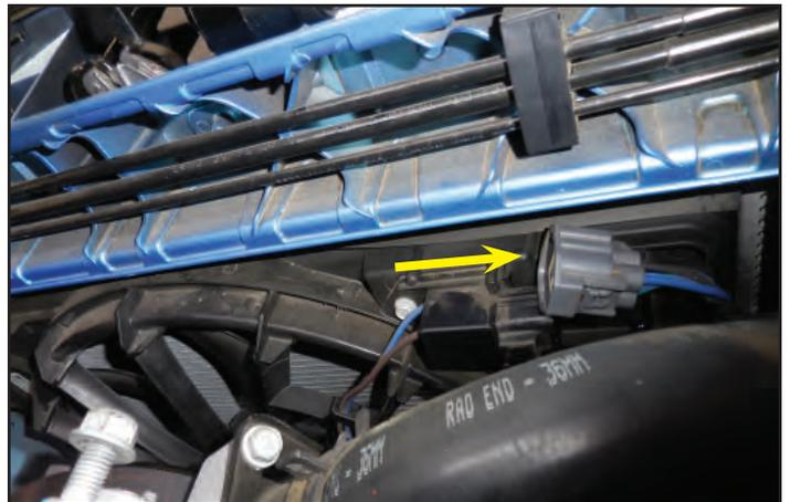
55. Remove the 10mm bolt securing the A/C line bracket to the vehicle in the location shown. Rotate the bracket out of the way to provide additional access to remove the fan shroud.
