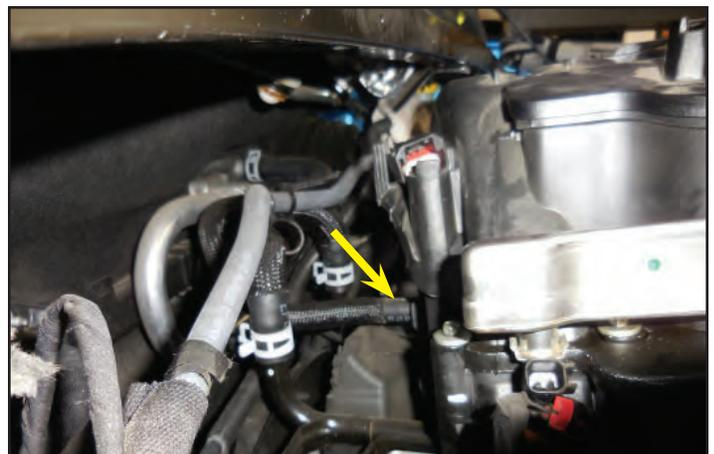
45. Carefully lift the OEM intake assembly from the vehicle.
