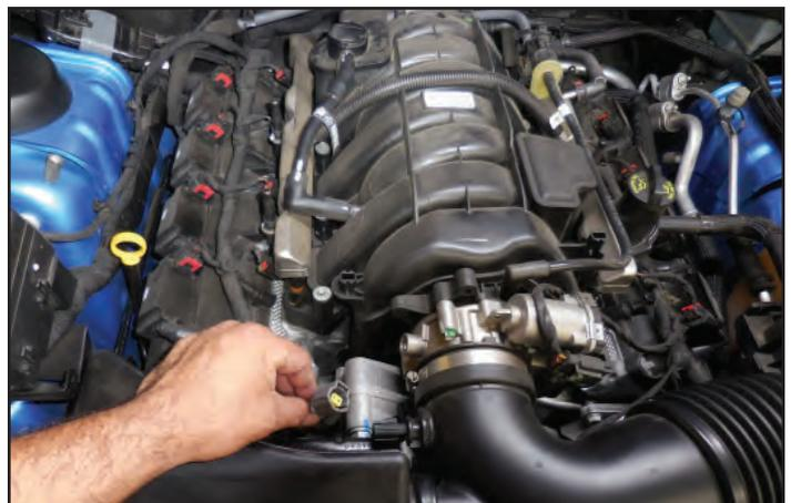
33. Loosen (2) gear clamps securing the clean air tube to the throttle body and airbox. Remove the clean air tube and airbox. Set them aside.
