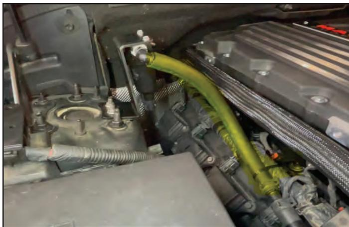
152. Install a 21mm constant tension clamp onto the end of the remaining ½” bulk hose. Install the end of the hose onto the PCV valve at the RH rear corner of the supercharger. Secure the hose using the clamp.
