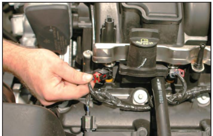
37. On the very back of the OEM intake manifold on the passenger side is the MAP sensor. Disconnect this plug and the mounting push pin clip as well. Disconnect MAP and IMRC sensor plugs @ rear of intake.
