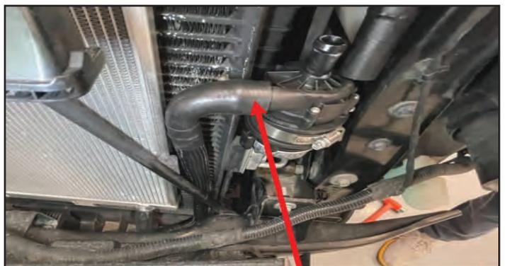
Secure the hose with a gear clamp @ pump and a constant-tension clamp at the LTR
