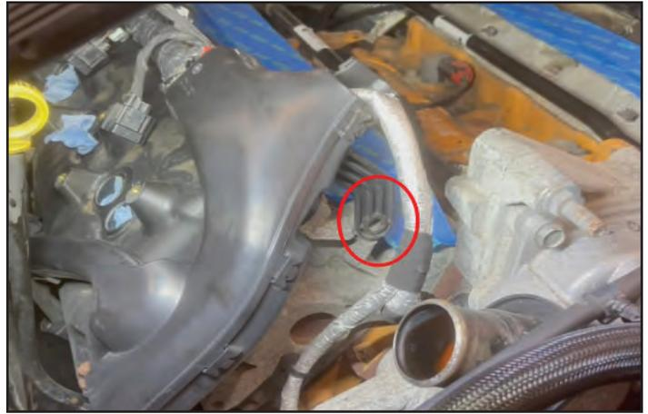
74. Select the low temp radiator (LTR) from the kit. Remove the Allen head plug from the top of the LTR. Select the 90-degree brass fitting from the kit. Apply thread sealant to the fitting threads. Install the fitting into the LTR by hand until slight resistance is felt. Then tighten it an additional turn followed by additional clockwise rotation to orient it as shown in the photo.
