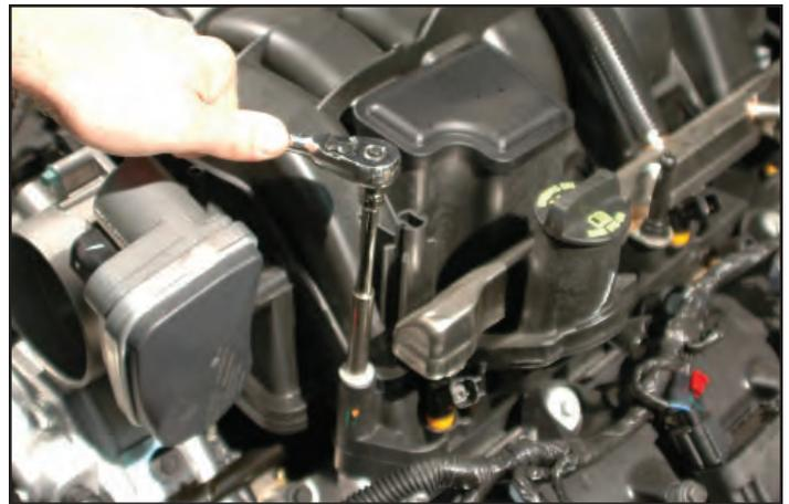
44. Pull the OEM intake manifold forward a bit to gain access to the brake booster hose plugged into the back of the manifold. Disconnect this hose from the rear of the intake manifold. There is also a wire loom clamp located at the back of the intake manifold that needs to be pulled free or cut off.
