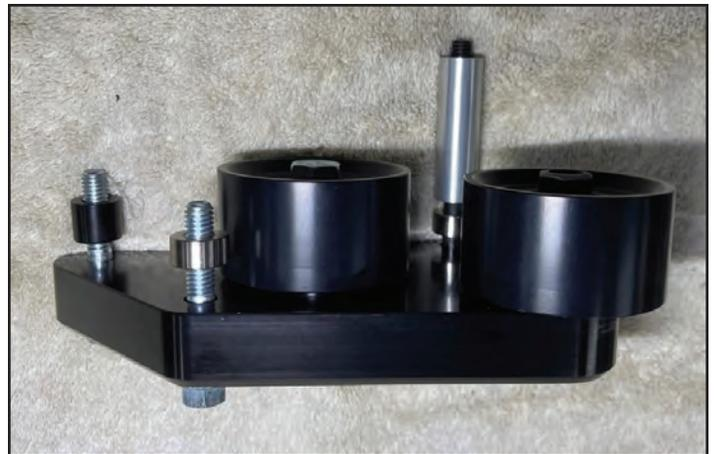
112. You will find an assembly drawing of the FEAD Idler bracket assembly at the back of this manual. There is one for 2009-2010 model years and another for 2011+. **Torque the idler fasteners 18 ft-lbs.**
