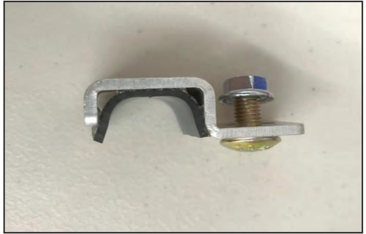
78. Pre-install both bracket sub-assemblies over the top of the A/C condenser core in the locations shown.
