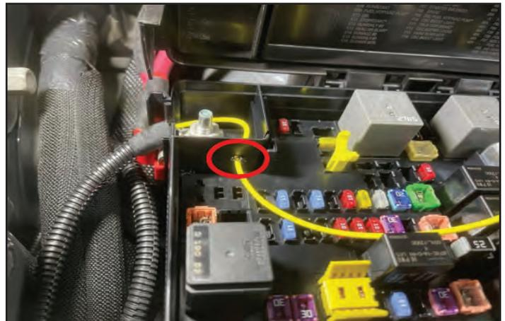
99. Remove the fuse from location F66 and install the copper tap that is crimped onto the end of the yellow wire. Re-install the fuse back into location F66.
