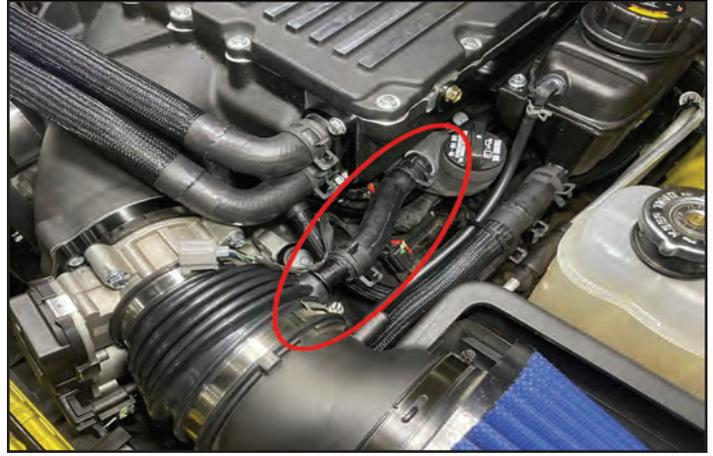
174. If your vehicle has a Mopar cold air intake kit installed, install the 1/2" rubber plug onto the air box fitting in the location shown. Note: cold air kit upper lid that fastens to the underside of the hood must be removed (insufficient clearance to supercharger)
