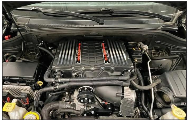
197. After the initial test drive, gradually work the vehicle to wide open throttle runs. Listen for any engine detonation (pinging). If engine detonation is present, let up on the throttle immediately. Most detonation is caused by low octane fuel still in the tank. **NOTE: PREMIUM GASOLINE FUEL MUST BE USED, 91 Octane or better.** If you have questions about your vehicles performance, please check with your installation facility.
