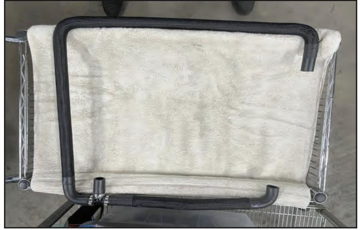
166. Install the hose assembly onto the charge air cooler upper ports as shown. Secure the hose using 3/4" constant tension clamps.
