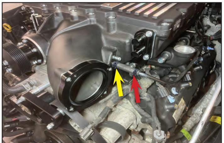
141. Re-connect the fuel line to the fuel rail on the LH side of the supercharger. Ensure the connector is fully seated, you will hear it click into place. Cycle the red lock on the connector. Pull back on the connector ensuring it does not come off.
