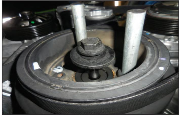
58. Use a pry-bar or long heavy duty screwdriver to anchor the pulley using alternate sides of the dowels you pushed in the pulley holes as shown. This will give you a lever to stop the pulley from turning. Now, use a 21mm wrench to remove the crank harmonic balancer pulley bolt. Set aside for later use along with the two provided dowels.
