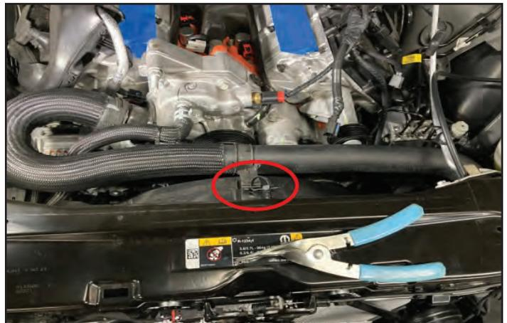
53. Disconnect the upper radiator hose from the water pump and move the hose out of the way to gain access to the front of the engine.
