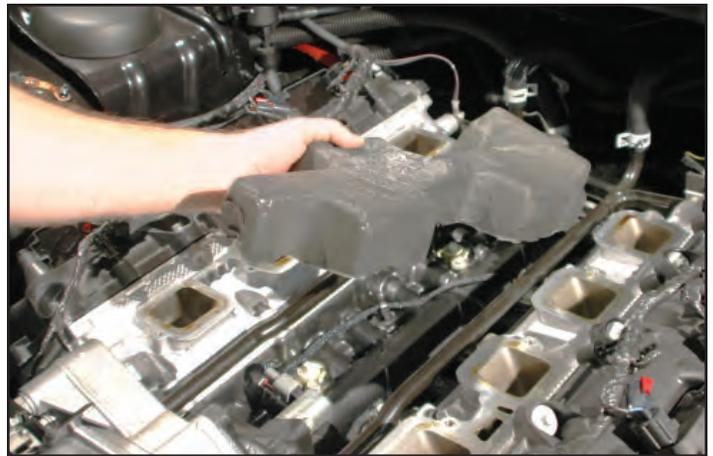
47. Use a vacuum to remove any debris from the heads and adjacent surfaces. Be careful to not allow any debris into the open ports.
