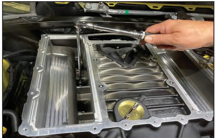
136. Re-install the charge air coolers into the supercharger ensuring the coolant ports line up with the holes in the front of the housing. **Apply blue Loctite 242 to (6) inboard CAC fasteners** and re-install them. **Torque them to 84 in-lbs.** Ensure the (4) black O-rings are in place as shown in the photo.
