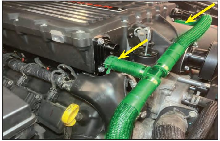
158. Route the opposite end of the 003C hose down in between the coolant reservoir and RH side of the radiator, then behind the pencil brace as shown highlighted in green.
