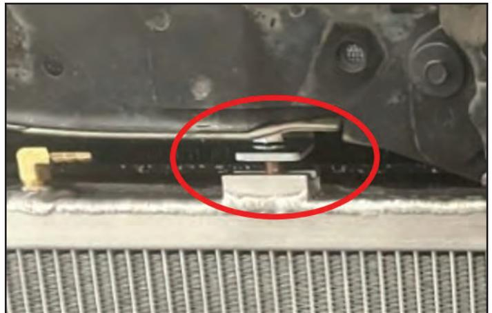
84. Rotate the factory pencil braces back into position so the upper holes align with the weld nuts. Mark the position on the LTR where the pencil braces intersect (RH side shown, LH side similar).
