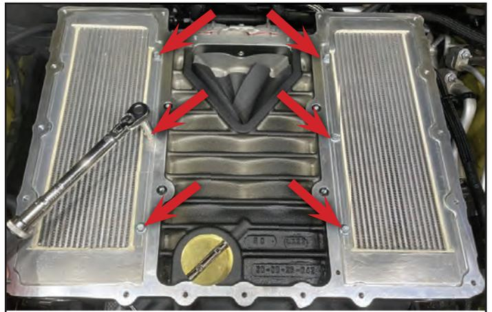
123. Remove (6) turret fasteners from the front securing the turrets to the base. Three fastener locations are shown here.
