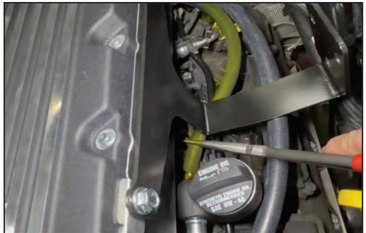
148. Select the U-shaped PCV hose shown in the photo. Install the long end onto the port below the bypass actuator. Cut the opposite end in the approximate location shown.
