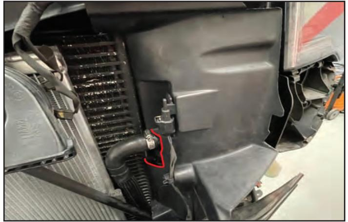
182. Re-install the front fascia reversing the steps found at the front of the manual. Push pins are provided to secure it in place where the original factory rivets were used.
