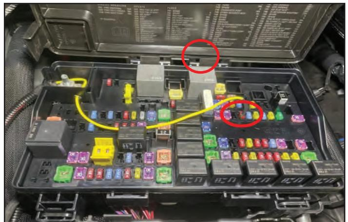
100. Remove the 13mm ground post and connect the BLACK ground wire to the base of it. Re-install the post and tighten it securely.
