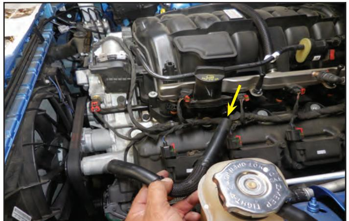
41. **CAUTION: Fuel line may hold residual pressure. Wear safety glasses to protect your eyes. Use shop towels to capture any residual fuel and dispose of it properly.** Remove the fuel line from the fuel manifold on the driver side. **For earlier models** you will press on the blue tabs of the fuel line locking clip and then pull the line free. For late models see the step below.
