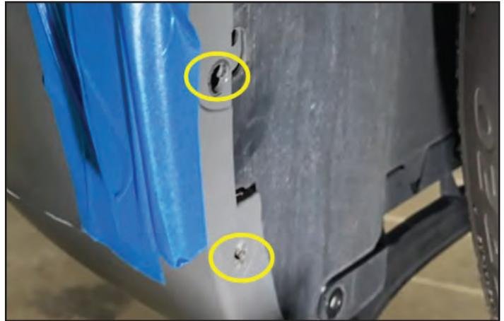
27. Working from underneath the vehicle, remove the fasteners, push pins and drill out any rivets securing the front fascia to the underbody panel.
