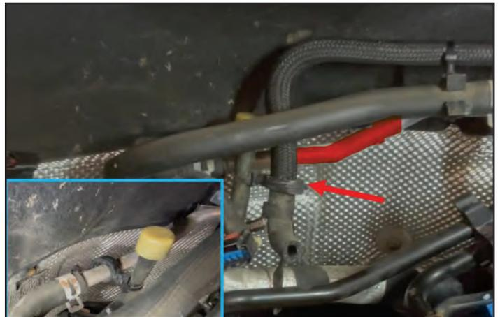
71. Remove the brake booster hose support clips from the heater hose (2 places) then cut the zip ties and discard the clips from the hose.
