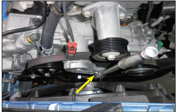
52. Remove the fir tree connector or lift and slide the tab securing the upper radiator hose bracket to the shroud.
