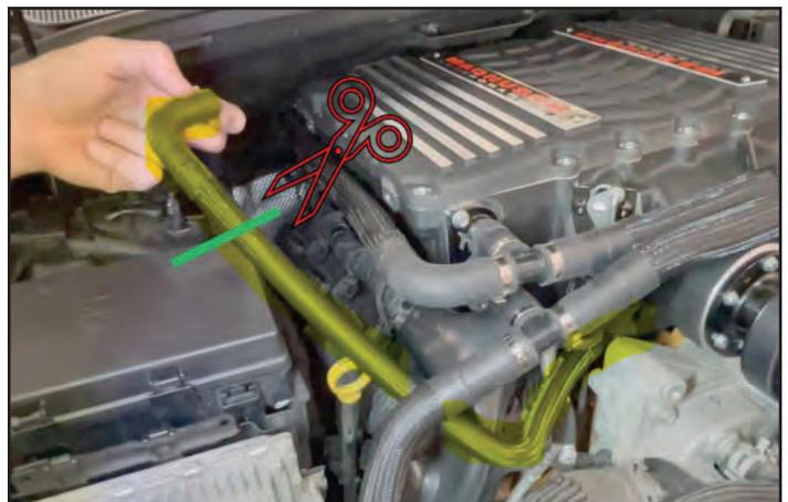
149. Install a ½” mender and 21mm constant tension clamp onto the end of the PCV hose as shown.
