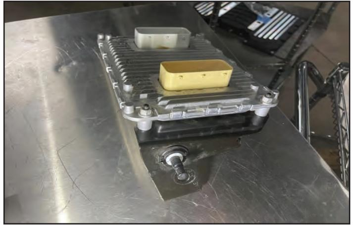
178. Re-install the PCM / bracket sub-assembly back in the RH side of the cowl. Re-attach both PCM connectors and the hood latch sensor connector.
