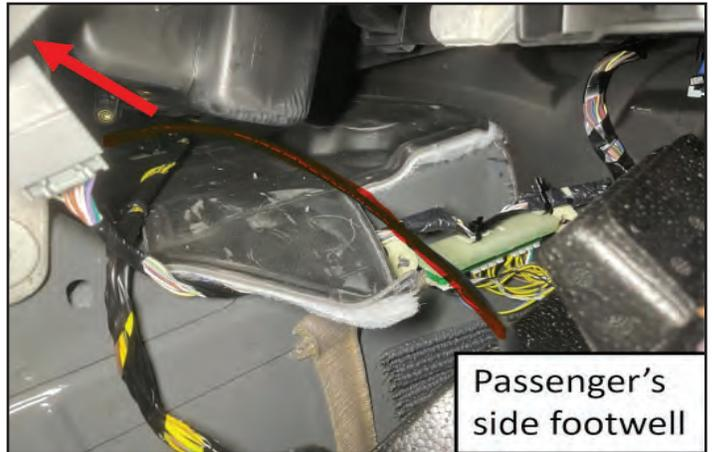
15. Working from the drivers footwell, route the connector above the drivers' side close out panel and over to the factory-installed OBD port.
