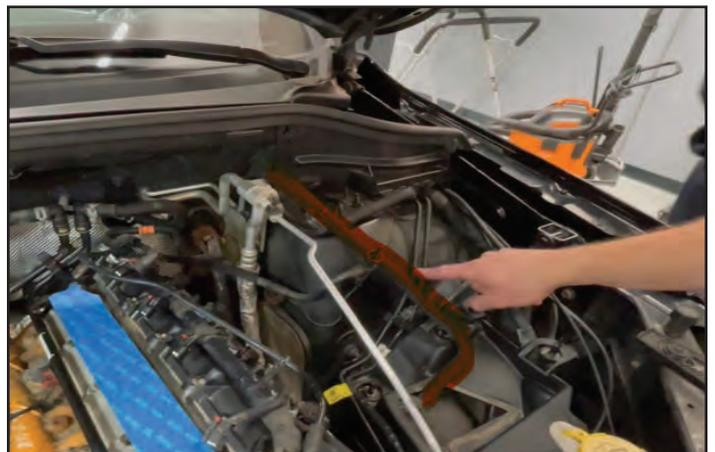
73. Remove the push pin that secures the black plastic bracket to the RH cylinder head in the location shown.
