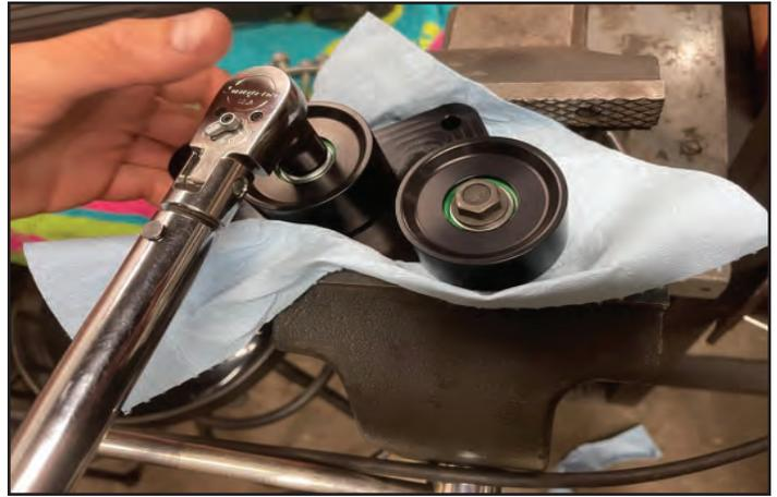
106. Remove the tensioner from the front of the engine using a 16mm socket.
