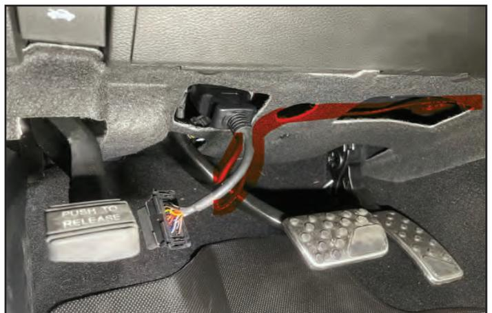
17. Back on the passenger side, connect the 2-pin plug into ANY open slot in the CANBUS connector. Ensure it is fully seated.
