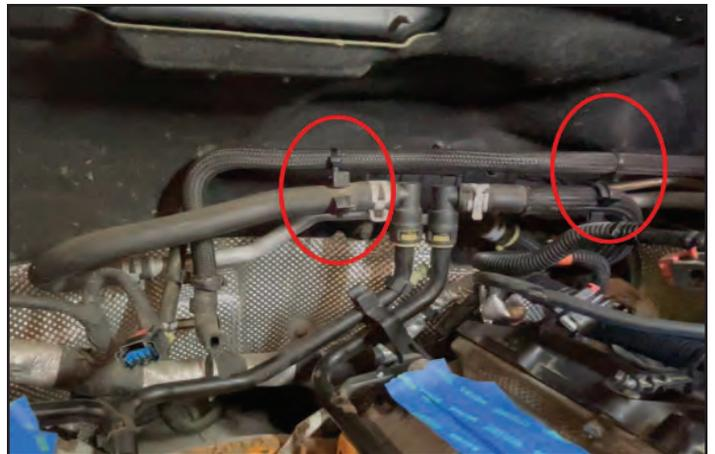
72. Temporarily stow the brake booster hose along the LH side of the engine bay. It will be connected in the later step.
