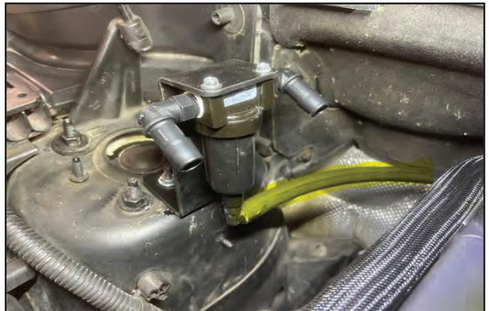
147. Route the opposite end of the hose around the back of the supercharger and over to the barbed fitting at the back of the oil fill adaptor as shown. Cut the hose to length and install it onto the fitting.
