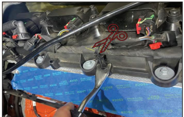
133. Remove any material covering the intake ports. Ensure they are wiped clean and no foreign material has entered the engine.
