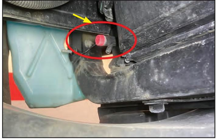
26. Inside the LH and RH front wheel wells, remove fasteners or drill out the rivets (as applicable) securing the front fascia to the fender liners and fenders.
