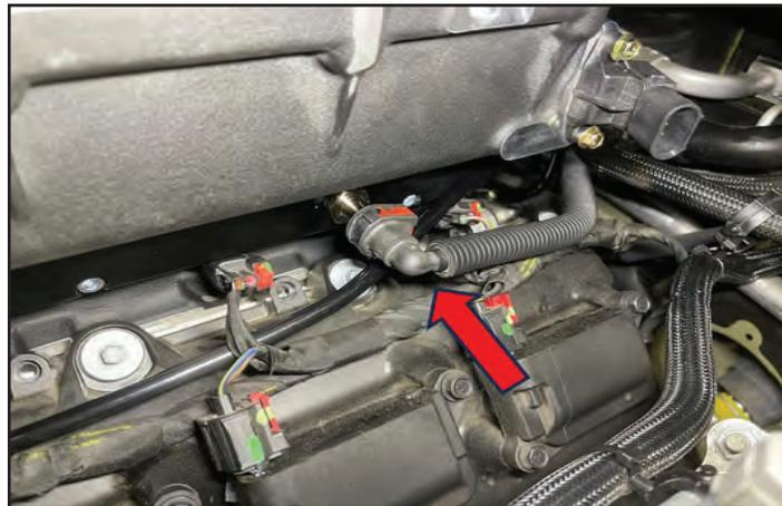
142. Route the factory brake booster hose around the LH side of the supercharger. Install it to the upper port on the supercharger behind the throttle body. Secure the hose with a 3/8" constant tension clamp at the circled location. Secure with a Zip tie the hose as required to secure it in place.
