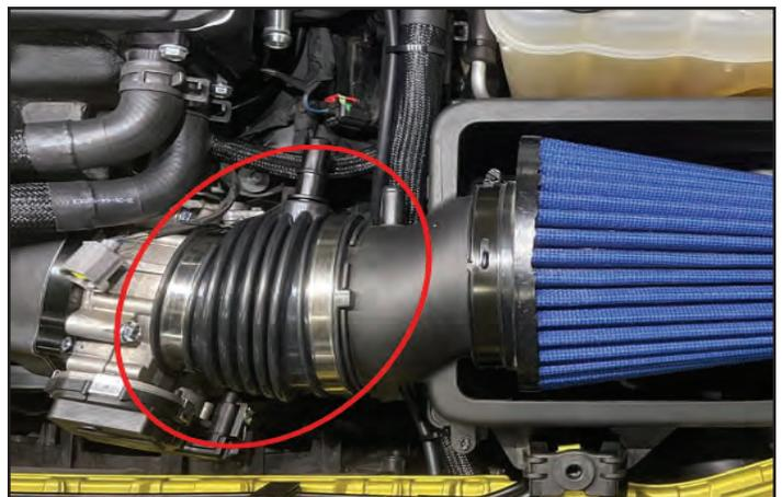
173. Install the 6 inch long piece of 5/8" I.D. rubber hose between the clean air tube and the oil fill adaptor for Mopar cold air intake. Secure the rubber hose using (2) 5/8" constant tension clamps as shown.
