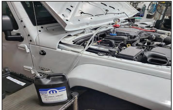
187. Pull a partial vacuum on the system and close the vacuum line.
