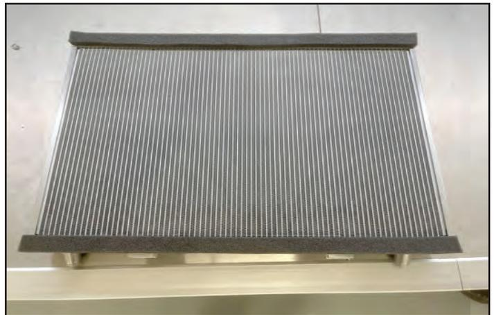
76. Cut and install adhesive-backed rubber isolators PN 68-01-00-049 onto the (2) short brackets PN 65-23-64-009 as shown.
