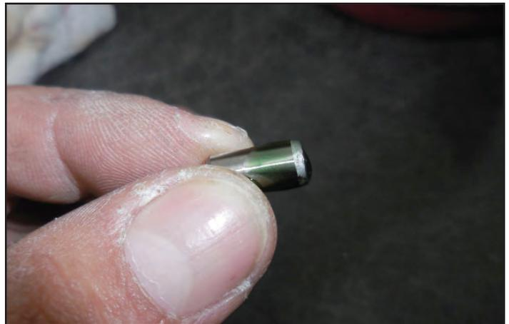
67. Use a hammer and drift-pin or nail-set to tap the crank pins in completely. Ensure that they are in completely, and will not touch the surface of the crank bolt directly when installed.
