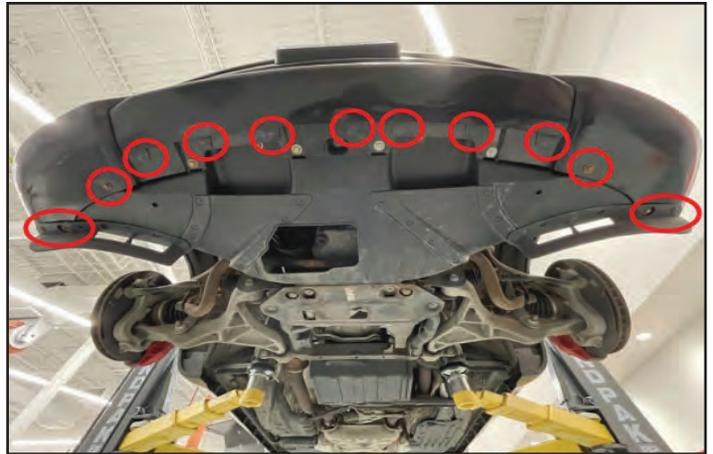
28. Remove the push pins located at the top of the fascia then pull up on the plastic panels to release them from the core support.
