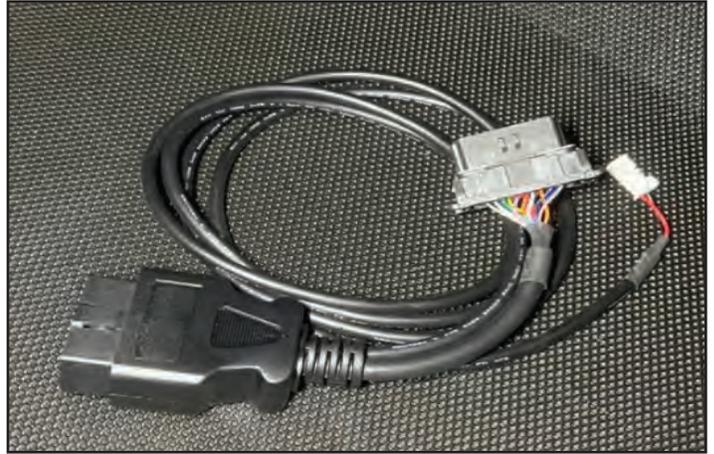
14. Pass the large OBD connector end of the cable through the center tunnel toward the drivers' side footwell.
