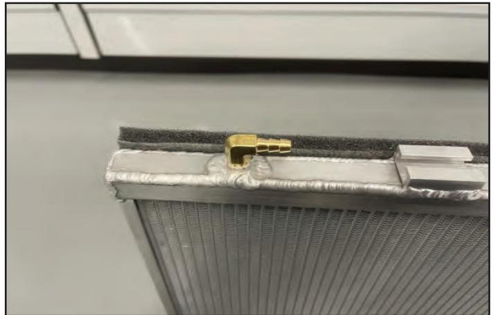
75. Select the self-adhesive foam tape from the kit. Cut the foam in two 23-inch lengths so it spans across the back of both the upper and lower tanks of the LTR. Apply acetone or brake cleaner to a rag and clean the tank surfaces so the adhesive will stick. Peel and affix the foam strips to the back side of the LTR on the upper and lower tanks as shown.
