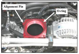
**4.** Install the supplied o-ring into the groove on the Airaid Spacer. Next install the spacer onto the intake manifold with the o-ring facing up, making sure that the alignment pin holes are located over the alignment pins.
