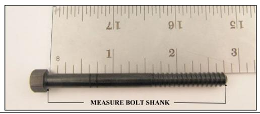
3. Measure your OEM hardware to determine which Airaid bolts you will need. Measure the shank only. Use the chart below to select the proper bolts.
