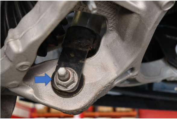
Step 19b. (Torque nut to 124 Ft. Lbs.)
