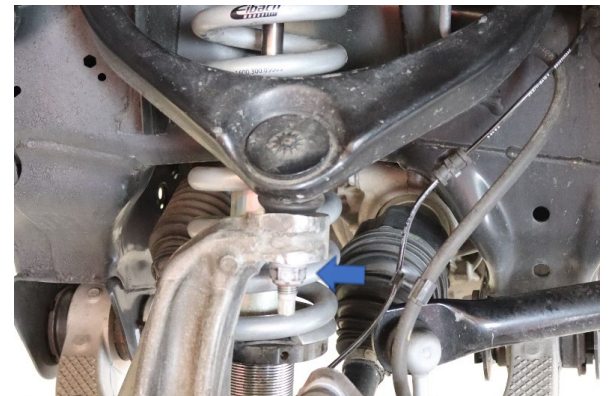
Step 22b. (Torque nut to 26 Ft. Lbs. + 180°)
