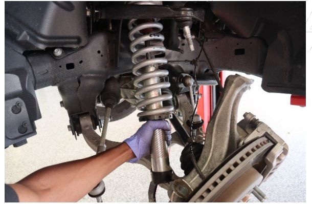
Step 16. Install new Eibach Coil Over shock
