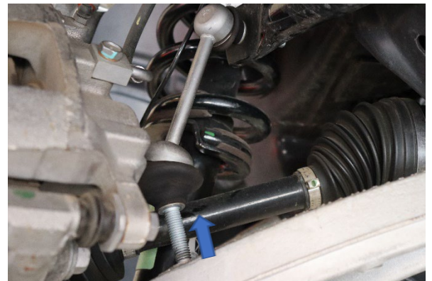
Step 9. Rotate the sway bar and lift the stabilizer link out of the lower control arm.
