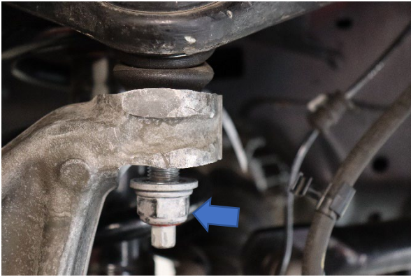
Step 4. Loosen the upper ball joint nut.
