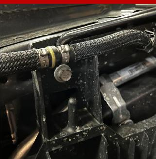
2. Use a 13mm socket to remove the bolt located on the passenger side of the engine bay. Install catch can and bracket in this location and reinstall bolt to secure the can in place.
