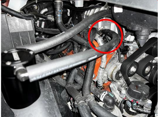
4. Install Hose A to the A side of the catch can and route the hose to the BLACK fitting on the engine. Make sure all fittings are secured in place and hose is pushed all the way over the barbed ends of the fittings.
