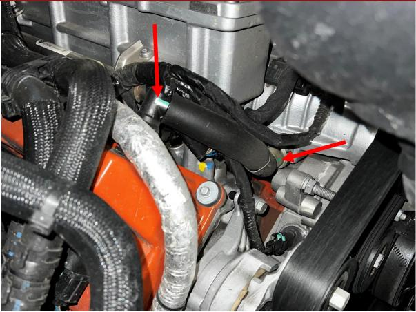
1. Locate the factory PCV line underneath the air intake on the passenger side of the engine. Remove the factory PCV line by pressing on the tabs on the quick disconnect fittings and pulling.
