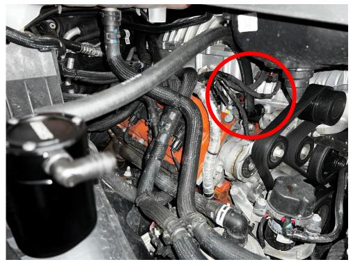
3. Attach quick disconnect elbow fittings to one end of each of the provided hoses. Install Hose B to the B side of the catch can and route the hose to the SILVER fitting on the engine. Make sure the hose gets routed ABOVE the 2 wiring harness lines to avoid potential contact with the supercharger pulley.
